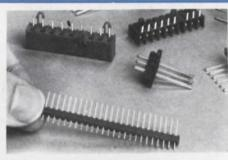
NEW FAMILY OF MINIATURE TERM-ACON SERIES CONNECTORS will solve majority of PC board interconnect problems. Moderately priced reliable designs for .100", .200" and .156" center pin spacings for hi-density to general purpose usage. U/L flame retardant Nylon material conforms to MIL-STD-202E. Polyester 94V-0 rated connectors are also available. METHODE ELECTRONICS, INC., 1700 Hicks Road, Dept. PR, Rolling Meadows, Illinois 60008. (312) 392-3500.
