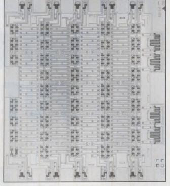
**Typical of uncommitted digital arrays,** this MasterMOS Model S chip contains 106 p-channel and 106 n-channel transistors, 10 medium-power buffers, four large n-channel devices with high-current capability, and one p-channel and one n-channel high-impedance device. The chip is  $65 \times 74$  mils, with pads of  $4 \times 4$  mils.
