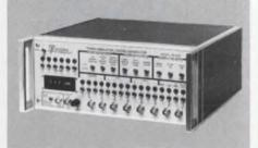
**RS-648 Timing Simulator/Word Generator** is intended for lab use by engineers and technicians who are debugging dgital circuitry or for production testing. It provides eight output channels and 16 memory words and is programmable to allow users to simulate exactly the desired timing signals or data transfers needed for device test. From Interface Technology, 852 North Cummings Road, Covina, CA 91724. (213) 966-1718.
