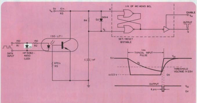
1. An optically coupled data-line receiver input uses a LED to protect the optocoupler unit from overloads. Also, the LED shows a visual flash when data are being received.
