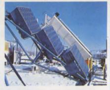
This two-axis, three-section tracking concentrator generates  $300 \text{ W}_p$ , and uses a solar-powered  $\mu$ P and stepping motors to follow the sun. RCA expects this "fly's eye" concentrator to cost \$1/W<sub>p</sub> in volume quantities.
