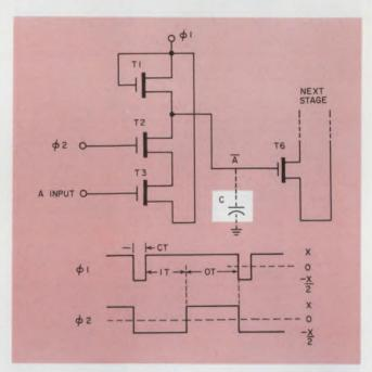
1. In a four-phase inverter, the inherent small capacitance of the next stage's input charges during time CT of clock  $\emptyset$ 1. The state of this capacitance is determined, during the input time (IT), by the condition of the logic input A. During the output time (OT), the output—the state of C—transfers to the next stage.
