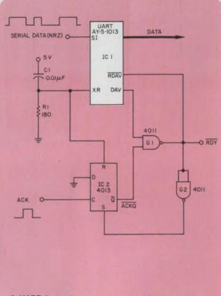
A UART in a simple handshake configuration can use the UART's double-buffer capability to speed data-handling throughput.
