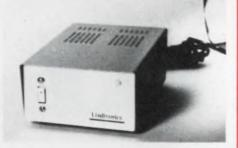
**TRIPLE OUTPUT REGULATED DC SUPPLY** — compact DC supply ideal for microprocessor and memories, Model 477-3 supplies 5V @ 500 ma,  $\pm 12V$  @ 100 ma and -5V @ 200 ma regulated outputs, input 110V 60Hz, the unit is enclosed in a compact steel case and complete with AC line cord with fuse. Unit price \$24.00. Lindtronics, P.O. Box 1792, North Brunswick, N.J. 08902.
