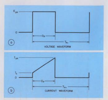
**1.** A trapezoid of current (a) results when a square wave of voltage (b) is impressed on an inductor. The initial jump of current,  $I_c$ , ramps up to the final value,  $I_{pk}$ , with a slope that depends on coil inductance and resistance.
