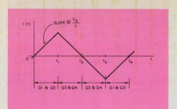
3. **Instantaneous current in a servo motor** is a triangular waveform whose average value is zero. Pairs of switching transistors in an SSA's power amplifier drive current to the motor through a fixed inductor to generate a triangular waveform.
