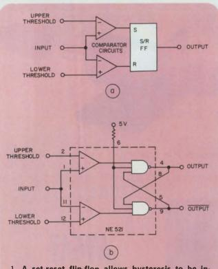
1. A set-reset flip-flop allows hysteresis to be introduced into a comparator circuit. And the threshold levels of the dead band can be set independently of each other.
