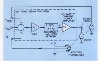
1. A complete servo amplifier is housed in a single switching servo amplifier (SSA) package. Depending on feedback elements, either a position or velocity servo can be built. In the SSA block,  $G_B$  represents not only the power-amplifier stage but also the control electronics section that provides drive signals.
