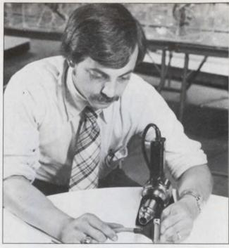
mold a shrinkable connector cover to a connector (right) without damaging the wires or connector. A clean flame or infrared can do the job in some cases.
