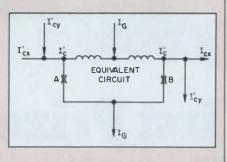
current  $I_G$ , and by two control lines that are inductively coupled to the cell. One control line,  $I_{cx}$ , is at right angles to the word line,  $I_G$ , while the other control line,  $I_{CY}$ , runs in a staircase pattern through a matrix of cells.
