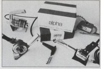
2. **Heating devices for shrinkable tubing** come in many styles and with a variety of attachments to provide uniform and rapid heating where needed.
