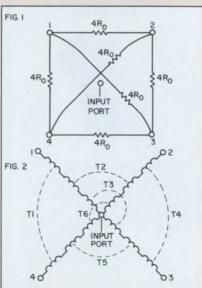
turns ratio (see Fig. 1). Each output port is connected to every other output port by a resistor of  $NR_o$ , so that the number of resistors required is 1/2N(N-1). N-1 transformer windings are connected in series between each output port and the input port, so that 1/2N(N-1) transformers are required.
