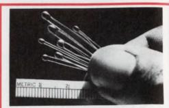
THERMISTORS with leads and coating are highly reliable low cost components in small dimensions more compatible with modern circuit design. R @ 25°C 100\Omega to 1 meg  $\Omega \pm 10\%$  to  $\pm 1\%$ . CURVE MATCHED INTERCHANGEABLES to  $\pm .25^\circ$ C. POINT MATCHED INTERCHANGEABLES to  $\pm .25^\circ$ C. Call or write for HP97 or TI SR52 THERMISTOR LINEARIZATION PROGRAM. WESTERN THERMISTOR CORPORATION, 354 Via Del Monte, Oceanside, CA 92054. (714) 433.4484.
