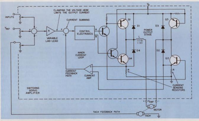
2. Motor drive in an SSA is provided by an "H" bridge. Alternate pairs of switching transistors,  $Q_1$  through  $Q_4$ , allow current to flow in the motor in two directions. An "H" bridge is a current source that senses current flow
