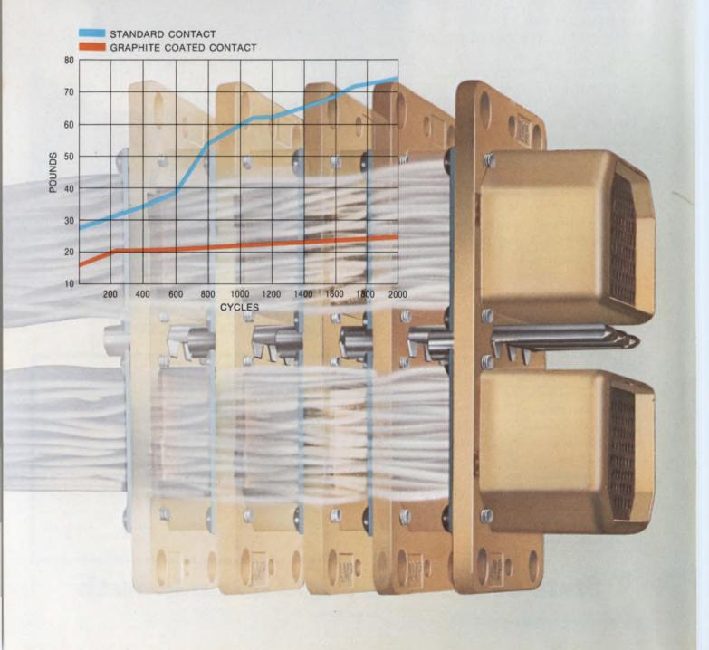
They give you all the advantages of lower insertion force without sacrificing proven contact geometries, or electrical stability. Insertion and extraction forces can be reduced as much as  $40^{\circ}_{e}$  which also results in extended contact life by more than  $100^{\circ}_{e}$ (as the table indicates).
