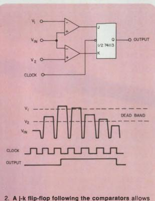
2. A j-k flip-flop following the comparators allows the circuit to be clocked to synchronize input data. In addition to hysteresis from the comparators, clocking helps reduce noise rejection even further.
