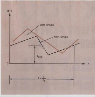
5. **Ripple current in a servo motor is a function of motor speed.** With constant frequency control, ripple current is large at low motor speeds, increasing motor heating. But current must circulate through a motor at all times to prevent a system dead zone.
