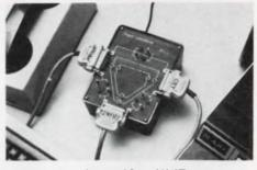
UNIVERSAL JUNCTION UNIT . . . for three devices, RS232C or current loop.
