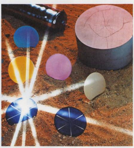
**Czochralski-grown silicon crystals** with up to a 5-in. diameter are sliced waferthin to produce solar cells. After diffusion, the discs are metalized with an electron-collecting grid. It becomes one of the output terminals. (Motorola).
