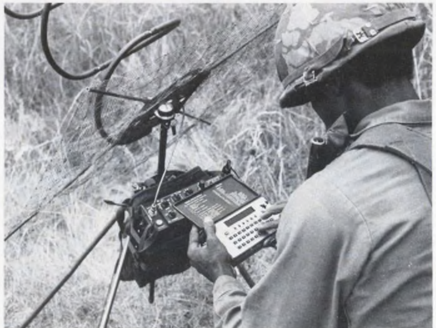
Using only 35 W of power and a satellite relay, the AN/PSC-1 can communicate with support units as far as 9000 miles away.
