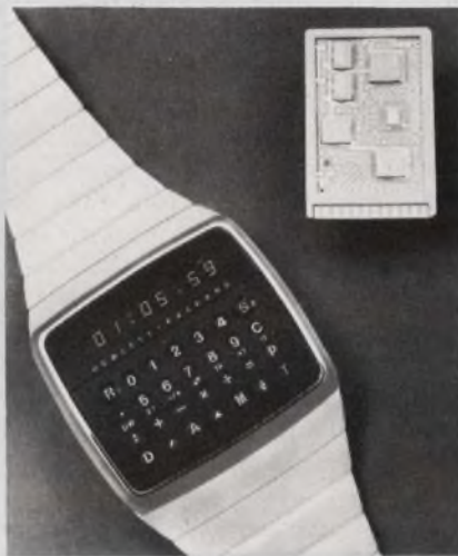
CMOS LED wristwatch contains hybrid with 38,000 LSI transistors.
