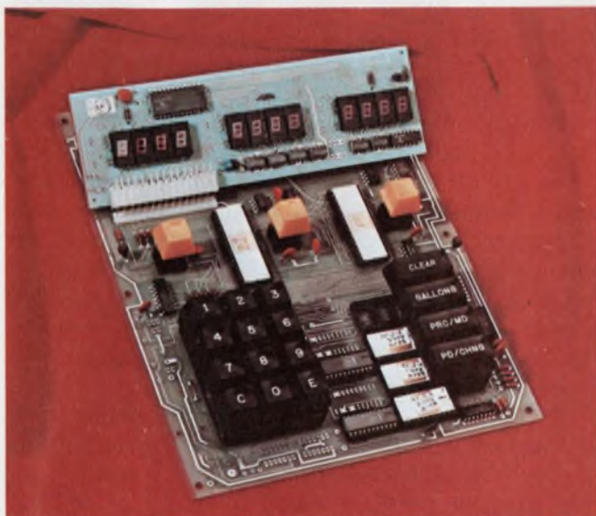
This self-service gasoline-station dispenser control system, by Bennett Pump Co., is an 8008A-based microcomputer that services a three-hose station module.
