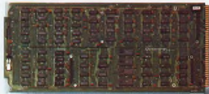
NAKED MILLI LSI-3/05 CPU, Type 1. Model 10300-01. Same as Type 0 at left, but also includes Real-Time Clock and AutoLoad capability.
