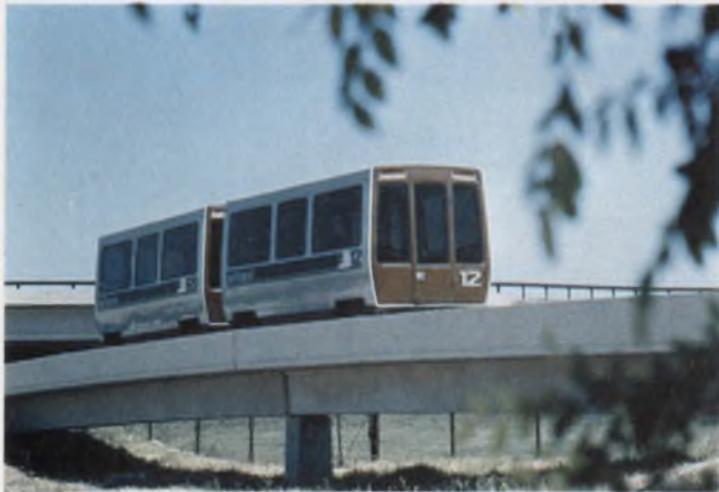
A hierarchy of computers runs Airtrans , Vought's total ground-transportation system at Dallas-Ft. Worth Airport. The master computer has 8 satellites.
