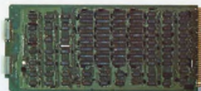
RAM-only Memories. Model 11642-XX. Choice of 4K or 8K words. Available with Battery Pack.
