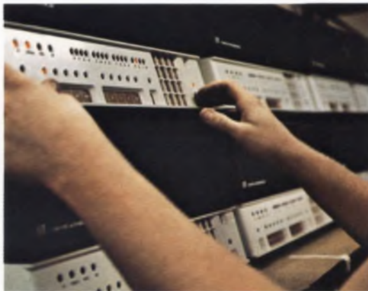
Computers awaiting shipment idle away the hours under test. Reliability benefits from the additional component aging.
