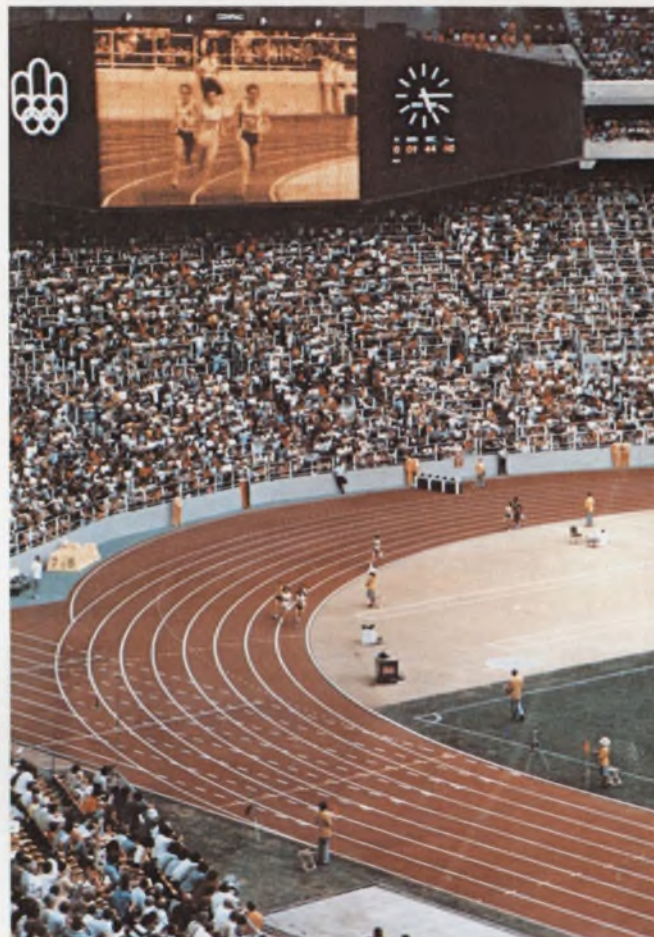
TV pictures and messages are flashed to Olympic Stadium spectators in Montreal on two computer-driven scoreboards designed by Conrac. Images from on-field and remote TV cameras are piped to 33 x 65-ft screens composed of 19,200 40-W incandescent lamps.
