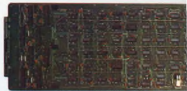
I/O Distributor. Model 14629-XX. In conjunction with Intelligent Cables (see text), the I/O Distributor provides up to eight interfaces—serial or parallel in any mix. Small version accommodates four interfaces. A DMA version allows data transfer rates up to 250K bytes per second.
