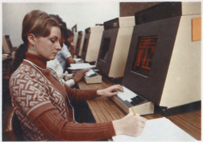
Terminals of Control Data's Plato university education system are designed around human interface requirements. A touch panel gives users access to the system.
