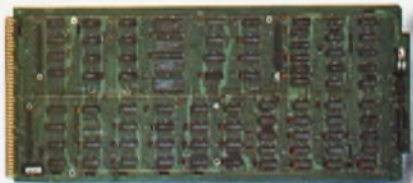
NAKED MILLI LSI-3/05 CPU, Type 0. Model 10300-00. Small low-cost processor offers exceptional power and features. 95 instructions, Power Fail Restart, vectored priority interrupts and 16-bit DMA port.
