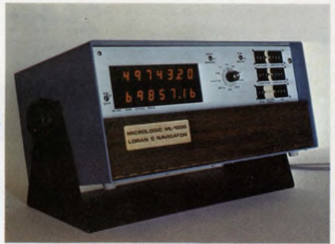
Two MCS-4 \mu Ps compute navigational functions in the ML 1000 Loran-C navigator by Micrologic of Chatsworth, CA. Piloting data are also provided.
