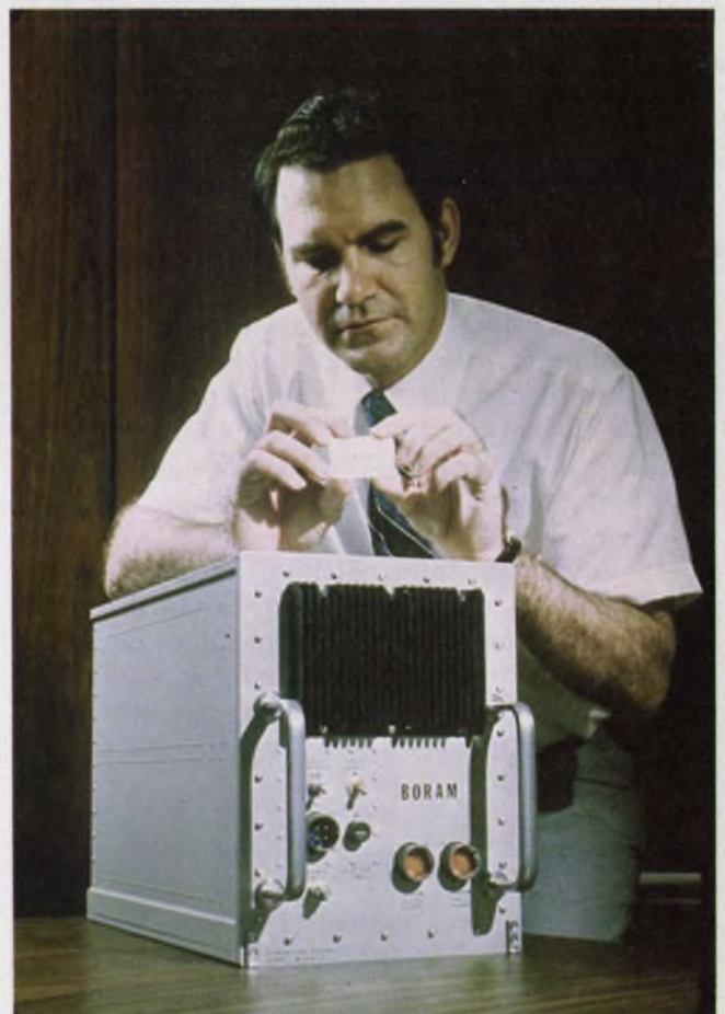
The Navy and Army have invested in Boram, a block-oriented, random-access memory that will store 16.8 Mbits of data (Westinghouse).
