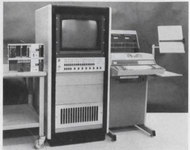
1. The over-all system with PACE on the left, mini and display-scope in the center and terminal at right.
