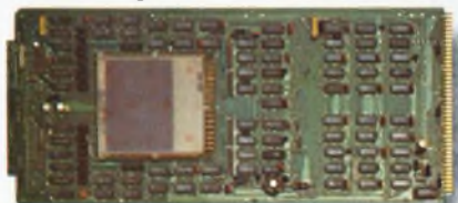
Half-card Core Memory. Model 11671-XX. 4K words. For either NAKED MILLI/ALPHA LSI-3/05 or NAKED MINI/ALPHA LSI-2 Series Computers.
