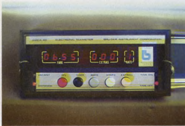
The \mu P-based taxi-fare meter easily accommodates rate changes with pluggable PROMs. The meter computes five fares simultaneously, permitting ride sharing.
