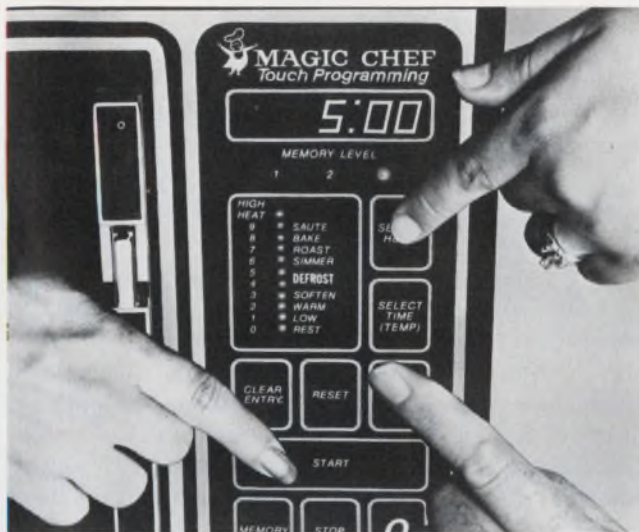
The newest microcomputer-driven microwave oven, by Magic Chef, has three pre-programmed memories that control independent timing and heating cycles plus associated displays.
