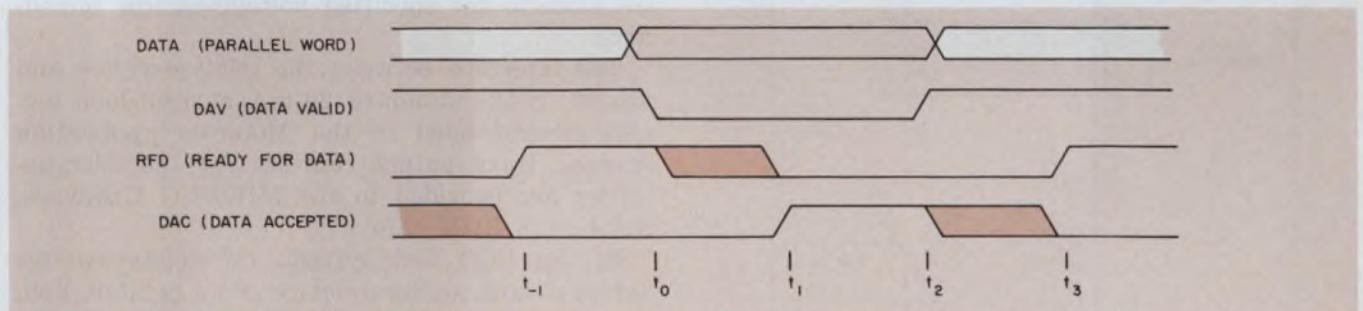
9. Transfer of data between the \mu P and the counter conforms to IEEE 488, the recently adopted interface stand-
