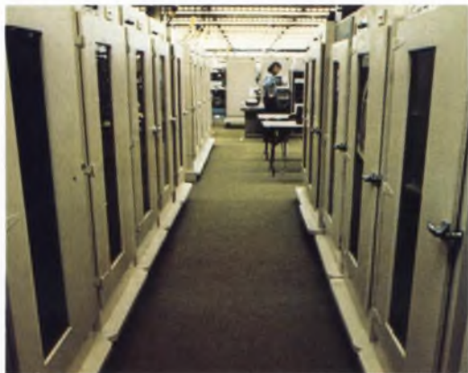
Temperature chambers stress computers to isolate marginal components. Computers are continuously tested during 72-hour burn-in at 50°C. Any error starts the test over from the beginning. To further stress the computer, power is cycled on and off approximately 2000 times during test.
