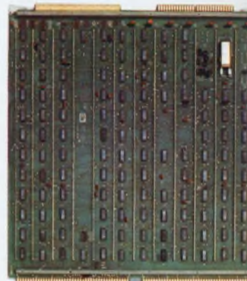
Magnetic Tape Controller. Model 14224-00. Provides interfaces for four 9-track standard tape units, or equivalent. Cabling separate.
