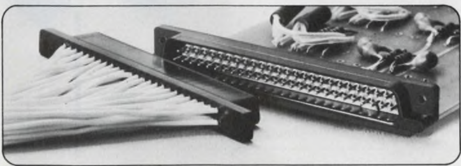
REAR VIEW ILLUSTRATES WIRE-WRAPPED TERMINALS
