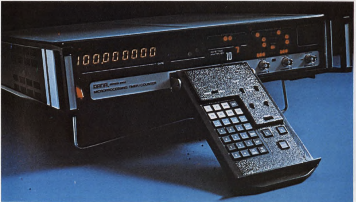
An instrument that can be interfaced to the IEEE 488 General Purpose Interface Bus is the Dana 9000. This
