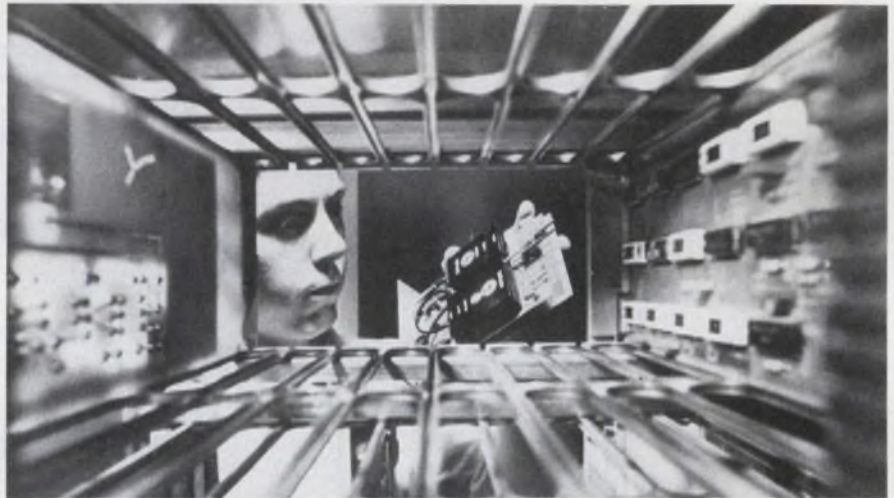
Circuit board containing experimental optical communications transmitter is removed from equipment bay. The lower black box contains the laser source; the upper box holds the control circuitry for the laser.
