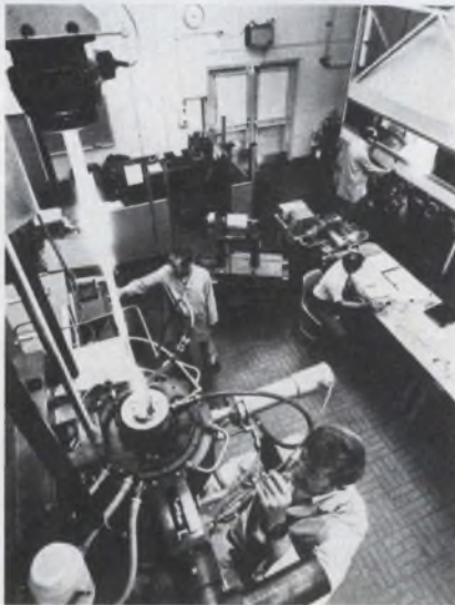
Glass rods are pulled into hair-thin fiber lightguides at Western Electric's Atlanta Works.
