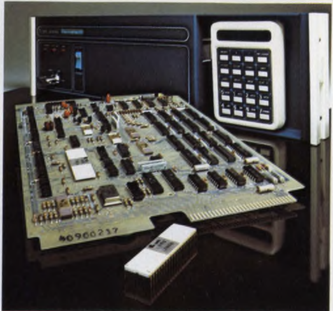
The packaging flexibility of a compatible microprocessor family, like the microNova, permits a relatively easy change in the level of processor or computer needed.
