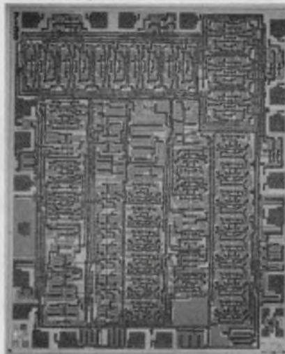
High-density CMOS CB-frequency synthesizer made by MicroPower Systems to Fanon/Courier's design.
