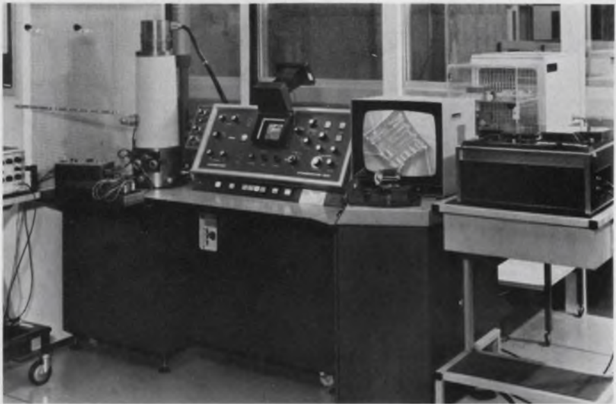
Microscopic flaws in LSI circuitry can be displayed and identified with the scanning electron microscope and TV-monitor system developed by the British Post Office. A video tape recorder preserves test records.
