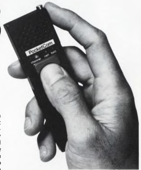
The PocketCom measures approximately 3/4" x 1 1/2" x 5/8" and easily fits into your shirt pocket. The unit can be used as a personal communications link for business or pleasure.
