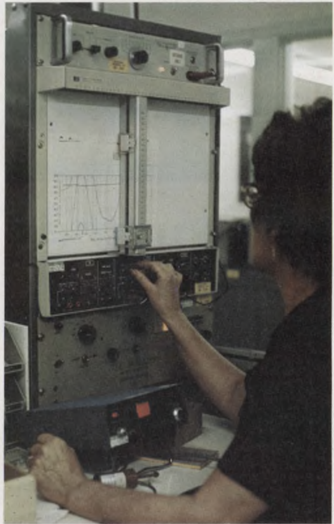
Crystal-characteristic data are obtained with instrumentation like that at Electronic Research. These data do not normally appear in data sheets, but can be requested.
