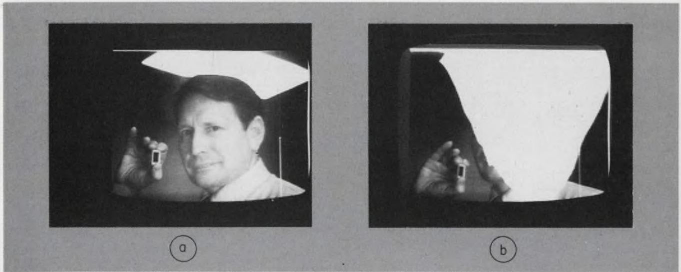
6. The improvement rendered by blooming control can be seen in RCA's 320 × 512 frame-transfer sensor (a).
