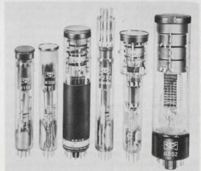
Phototubes from Hamamatsu such as these can produce gains of 100 to 100 million. Used for very low light level detection where good signal-to-noise ratios are important, their best sensitivity is at about 400 nm.
