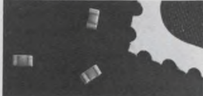
High-value thick-film resistor chips made by Eltec are so small that stamp perforations dwarf them.
