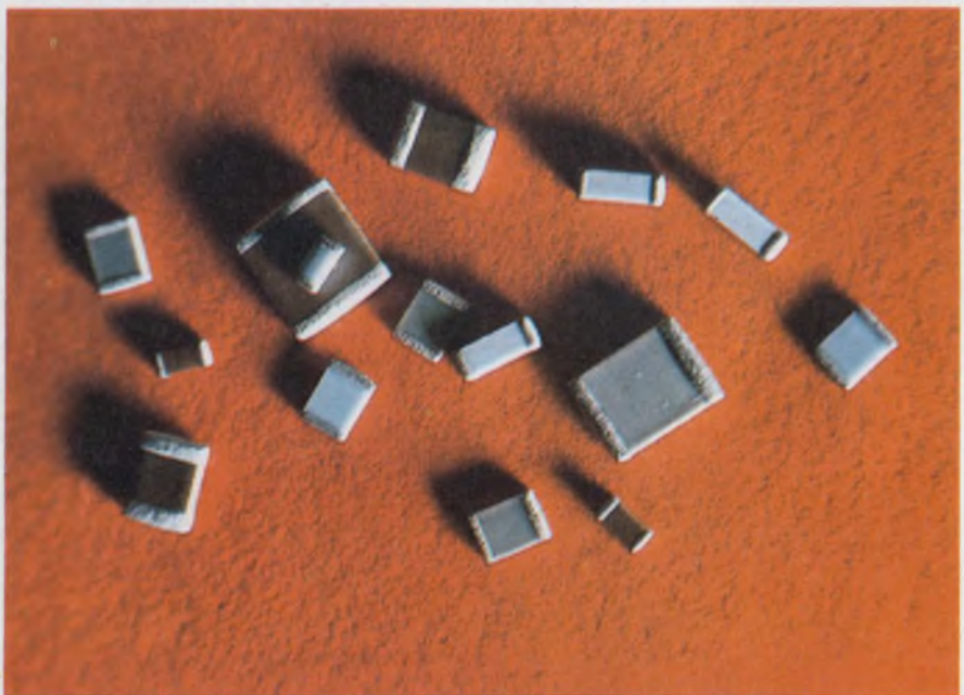
Ceramic chip capacitors in various sizes, including these from USCC/Centrolab, range in value from 0.1pF to over 200 \mu F. Ratings are from 4 to 200 V.
