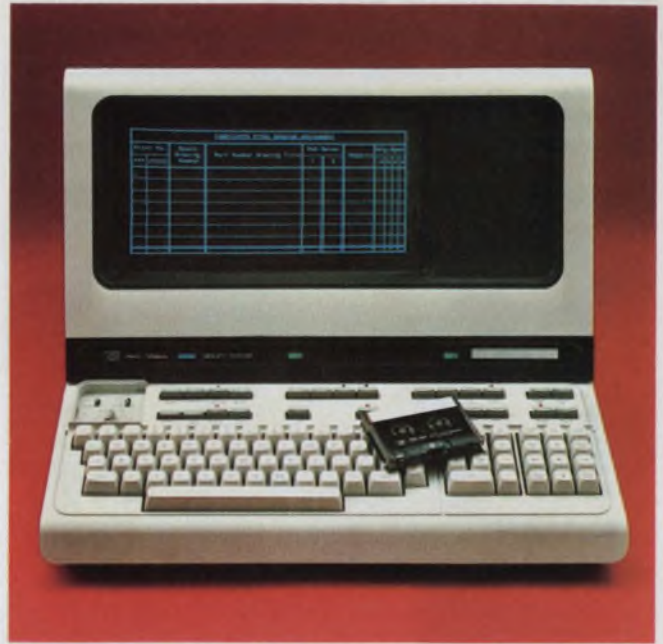
Omron's 8025 is a powerful intelligent terminal that is offered with an external programmer's console that facilitates debugging.
