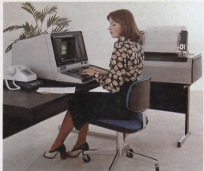
Sycor's 350 intelligent terminal contains a pair of built-in floppy-disc drives and a range of interfaces for other peripherals.
