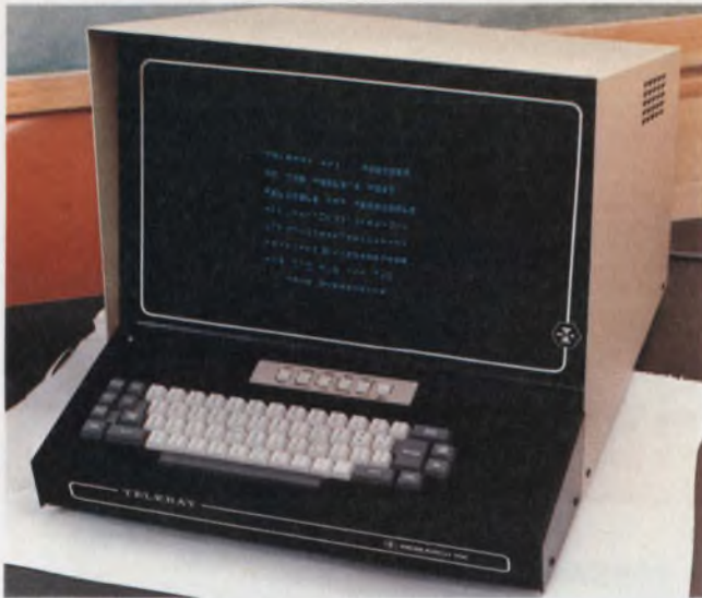
Research's Teleray 3900 is a terminal that provides APL as well as ASCII characters. A 15-in. CRT is used, and high readability is achieved.
