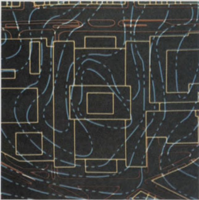
Conographics is the name given by Hughes to its technique of directly drawing curves for graphics rather than just straight vectors. This color display is from the Conographic-12 system.
