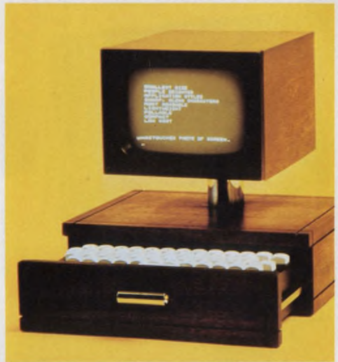
A compact 5-in. CRT and unusual styling with a keyboard in a drawer make this terminal from Informer unique in its field.
