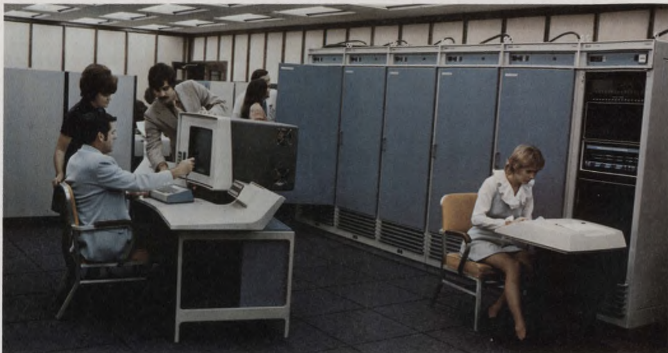
Together with multiple processing elements, this Staran S-1000 has a memory organized so that it can be ac-
