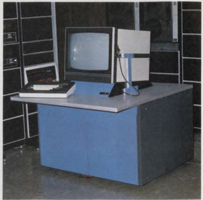
Lundy's 32/200 is an interactive graphics terminal in which the display is fully buffered and requires no overhead in the computer for refreshing the CRT.
