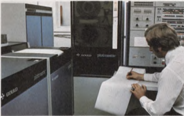
Electrostatic printers such as the Gould 4800 can print 3600 lines/min or draw complex diagrams and charts; and do it silently. The Gould 5200 has 200 styli/in. and
