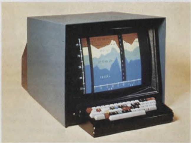
The Intecolor 8000 is the only single package, eight-color intelligent terminal available. The terminal comes with either the Intel 8008 or 8080 microprocessors and up to 24 k of RAM.
