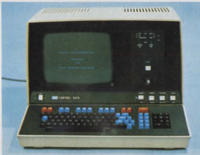
An Intel 8080 microprocessor is the heart of the Control Data 92451 Display Terminal. Control of the basic terminal is performed by semiconductor read-only memories mounted on PC boards within the terminal.
