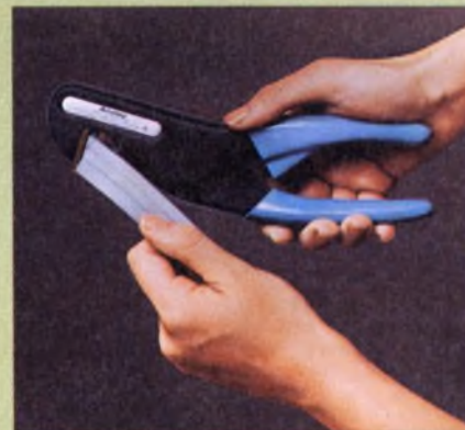
Pre-set compression cycle assures connection reliability.
