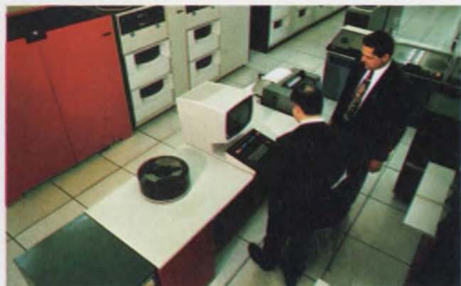
Distributed processing is found in the architecture of this IBM 370/125. Functions are assigned to I/O, arithmetic, and diagnostic processors.
