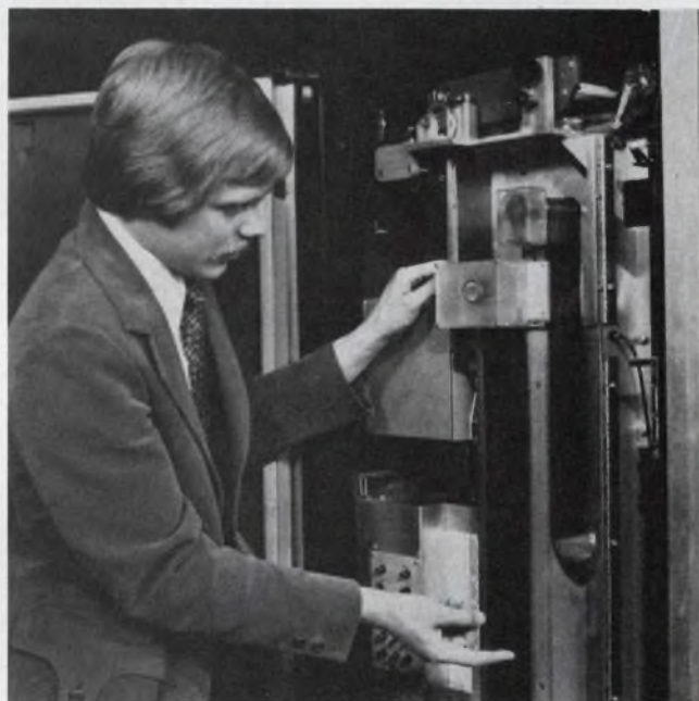
Data cartridges in CDC's 38500 mass memory system are read at a read/write station where the tape inside is automatically unwound into vacuum columns. Information is transferred at 806,000 bytes/sec.
