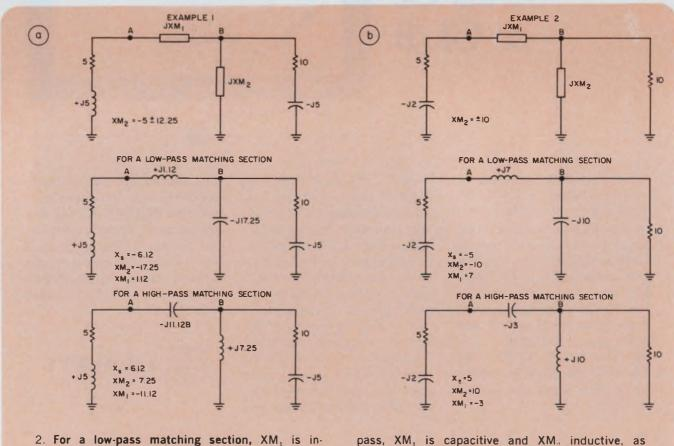
2. For a low-pass matching section,  $XM_1$  is inductive and  $XM_2$  is capacitive. However for high-
