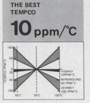
Self compensating characteristics are inherent in the proprietary Bulk Metal® process and produce a dome-shaped T.C. curve with a typical TCR of 5ppm/°C (absolute maximum TCR of 10ppm/°C for all values).
