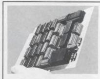
DIGITAL MATCHED FILTERS COR-RELATORS CONVOLVERS. Ltd. guan-RELATORS CONVOLVERS. Ltd. quan-tities Model 328 (32 word x 8 bit) and Model 2561 (256 word x 1 bit) correlators available. Also custom units built to order. Inputs: Two dig-ital signals, sampling/clock signals, 5V. Output: Correlation product. \$2/word x bit FOB ARO 90 days RCS ASSO., INC. (714) 624-1801. PROCESSOR 606
