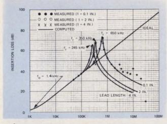
3. Computed insertion loss agrees closely with measured results, especially at the practical lead lengths.
