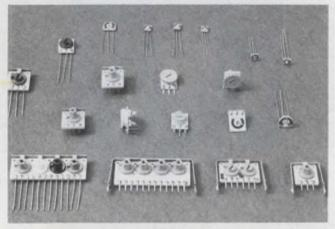
**Miniature trimming potentiometers** on ceramic substrates from Centralab permit the mounting of multiple units with just a single machine operation.
