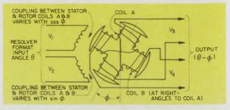
4. The resolver differential transmitter has two fixed coils at 90° to each other and two moving coils, also at 90° to each other. These moving coils determine the output of the unit in terms of the input angle and the shaft angle of the differential.
