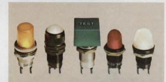
**INCANDESCENT OR NEON SUB-MINIATURE INDICATORS**—Meet or exceed MIL-L-3661. Mounts in 15/32", 1/2" or 17/32" clearance holes. Incandescent for 1.35-28V; neon has patented built-in current limiting resistor. Choice of cylindrical, faceted, convex, flat, square and round lens shapes, finishes, legends. Stocked by local distributors.
