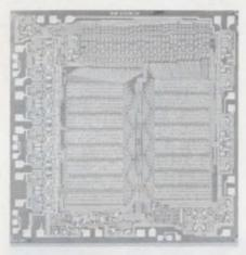
Static ROMs like this p-channel 4096-bit device from National Semiconductor use a low threshold voltage technology to achieve bipolar compatibility.
