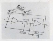
**Bipolar and MOS transistors are combined** on the chip of this highperformance sample-and-hold unit by Datel Systems. An external holding capacitor is used.
