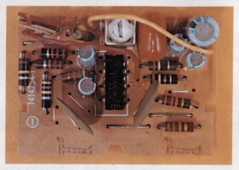
Stereo decoder printed circuit board contains an RCA 3090 phase-locked loop IC. These decoders are produced by the millions for use in home, auto and hi-fi FM radios.
