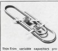
vide a reliable means of adjusting capacitance without abrasive trimming or interchange of fixed capac-itors. Series 9401 has high Q's and a range of capacitance values from 0.2-0.6 pf to 3.0-12.0 pf and 250 WVDC working voltage. Johanson Manufacturing Corporation, Boon-ton, New Jersey (201) 334-2676. THIN-TRIM CAPACITORS 601
