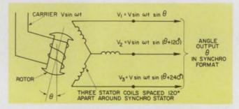
5. Synchro transmitters or receivers have three fixed coils that are spaced at 120° angles around a moving coil. The carrier signal on the moving shaft gets modulated and impresses signals in the three fixed coils that are 120° out of phase with one another.
