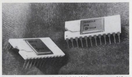
Three IC chips are mounted in this hybrid 12-bit current-output DAC by Analog Devices. The hermetically sealed device uses high stability, thin-film SiCr resistors. Laser trimming provides this AD563 with true 12-bit accuracy.
