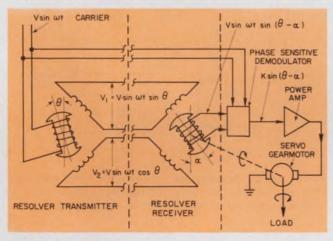
3. A simple resolver control system consists of a resolver transmitter, receiver, phase-sensitive detector and a power amplifier to boost the output.
