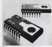
This monolithic, dual-channel power amplifier, by National, delivers 7-W per channel to an  $8-\Omega$  load. The device has overcurrent and thermal protection.
