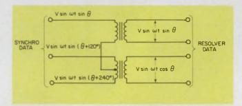
6. The Scott-T transformer changes the three-wire synchro signals into four-wire resolver-compatible data, or vice versa since the transformer is bidirectional.
