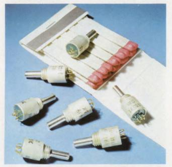
**Ultraminiature panel-mounting potentiometers** (Model 9917) from the IRC division of TRW require only 0.33 in. of behind-panel width and handle 0.5 W at 85 C.
