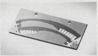
This quadrasonic joystick-panner control element made by Computer Instrument Corp. provides a 90° sine/ cosine function and has mechanical travel of 60°.
