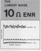
A multi-fingered precious metal alloy wiper in contact with the highly conductive surface of multiple resistance paths virtually eliminates both dynamic noise and catastrophic failures.
