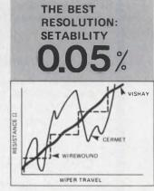
The Vishay Bulk Metal® process and the unique patented design assures an accurate setability of less than 0.05% regardless of value while wirewound technology ranges from 1.55% to 0.25%.
