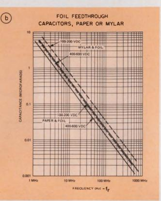
6. Self-resonant frequencies,  $f_r$ , for some types of feedthrough capacitors are dependent upon the capacitors'
