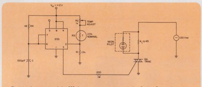
The internal comparator of the 555 timer, combined with a thermistor, makes a low-cost temperature controller. Resistor  $R_2$  sets the temperature trip point.
