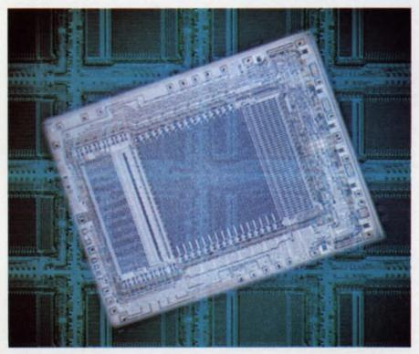
A field-programmable logic array has 16 inputs, allows 48 product terms and generates eight output functions. From Signetics, the FPLA employs fusible nichrome links as the programming elements.
