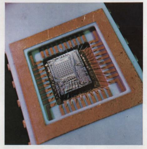
A 4-bit microprocessor slice, or microcontroller, has a cycle time of about 100 ns. The low-power Schottky-TTL circuit from Advanced Micro Devices can be used for minicomputer emulation.
