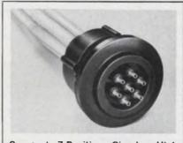
Compact 7-Position Circular High Voltage Connector. Military type LGH connector handles 15KVDC pin-topin or pin to ground. Can be her-metically sealed. Includes positive closure feature. Deeply recessed contacts. From the people with the most experience in high-voltage connec-tors. AMP Capitron Division, Elizabethtown, Pa. 17022. (717) 367-1105 **HV CONNECTOR** 612
