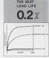
Only the Vishay Bulk Metal<sup>®</sup> element can provide a stability of 0.2% max. △R through a 2,000 hour load life.
