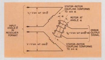
2. The electrical circuit of the resolver receiver looks identical to that of the transmitter, except that the roles of the coil windings are reversed.
