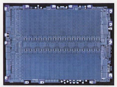
**SOS/CMOS memories,** such as this 1-k TA6780 from RCA, are challenging bipolar devices for applications where speed and low power operation are important. The device is now available in sample quantities.
