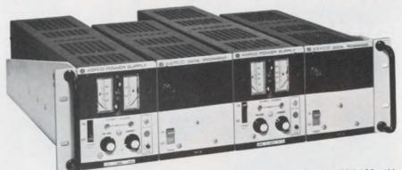
One power supply, Model JMK 100–1M produces 0-100 volts controlled in 12-bit binary; and 0-1 ampere controlled in 8-bit binary. The other unit, Model JMK 15–6M produces 0-15 volts controlled in 3-digit BCD; and 0-6 amperes controlled in 2-digit
