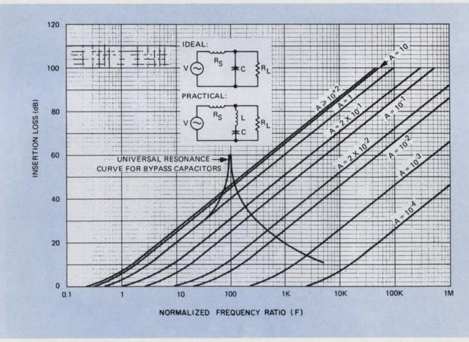
1. A family of normalized insertion-loss curves for idealized bypass circuits and a universal curve to correct for
