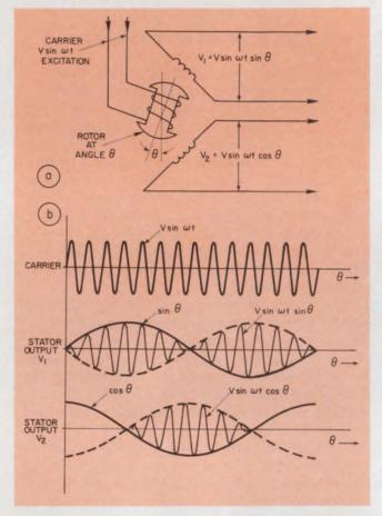
1. Coupling between the rotor and stator windings of the resolver transmitter varies with the sine and cosine of the shaft angle (a). The carrier waveform gets modulated by the motion of the rotor and the resulting variation in the coupling between the rotor and the two fixed stator coils of the resolver (b).
