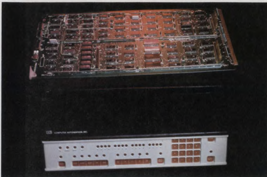
Computer Automation was the first with board-level minicomputers. The latest in the series is the Naked Milli LSI-3/05, which sells for only $295 as a CPU with no additional memory. Shown next to a full-scale Alpha LSI minicomputer, also made by Computer Automation, the Naked Milli is a bipolar minicomputer priced in the same range as board-level microcomputers.
