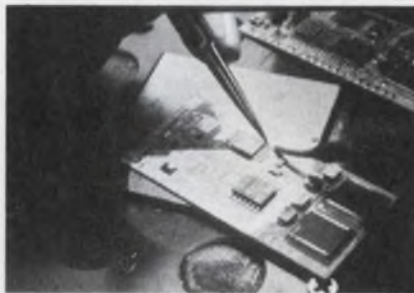
Some discrete components are still hand soldered to the hybrid's substrate, especially in small quantity and prototype designs.
