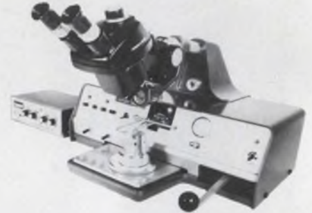
Motorized ultrasonic ball bonders, such as this Model 9700 unit offered by West Bond Equipment, provide the capability of presetting tool motions for repetitive action.
