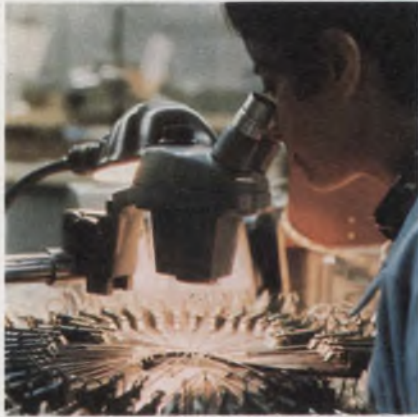
Probes are set up to test hybrid circuits at various stages in Raytheon's manufacturing cycle to detect defects before final encapsulation.
