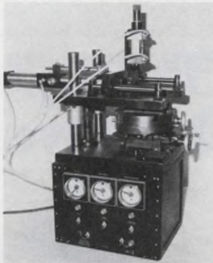
Aremco's 1975 version of its 3100 screen printer provides new squeeze pressure controls, settable timers, vibration-free motion and 0.0003-in. repeatability.
