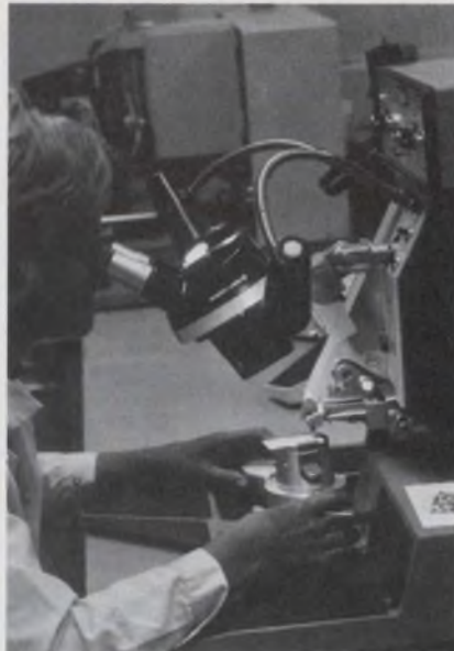
Bonders come in many sizes and forms. This bonder performs ultrasonic aluminum-wire bonding.
