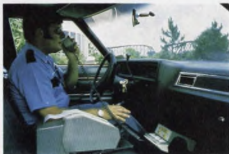
Computer-to-car communications system developed by General Electric expedites law enforcement. Officer in car (left) uses push-button console associated with radio control unit at dashboard to send predesignated digital messages to police dispatch center (right).
