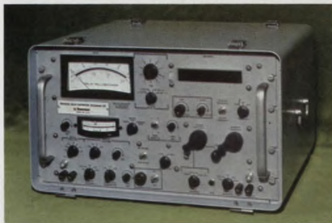
Envelope-delay distortion is particularly destructive to data communications. Bowmar's 490B transmission measuring set allows selection of a wide range of parameters to thoroughly cover modern data channels.
