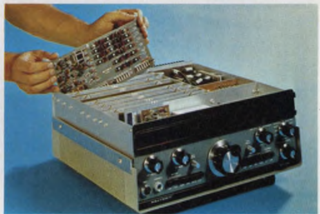
Broadband amplifiers simplify switching and tuning of both receiver and transmitter in this Heath SB-104 communications set.
