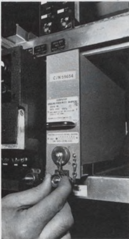
The ground proximity warning computer is the heart of the ground warning system made by Sunstrand.
