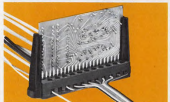
Models available for surface or through-the-panel mounting, with or without card guides and keys.
