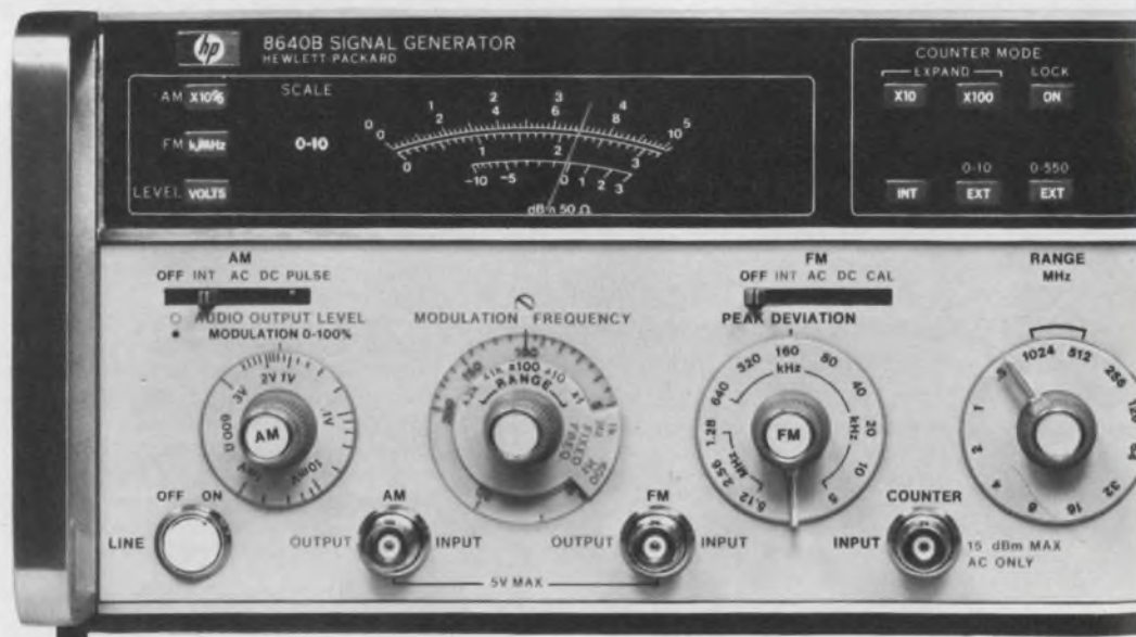
8640B with variable modulation, reverse power protection, and extended frequency options.
