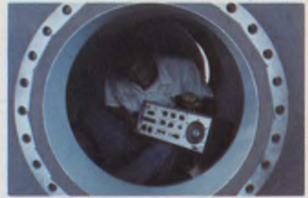
Helium speech unscrambler by Helle Engineering is brought out of a Perry Ocean Engineering personnel transfer bell for inspection.
