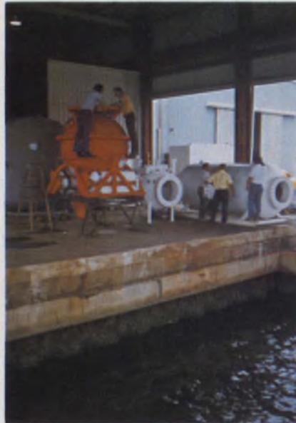
Pressurized "elevators" to take divers to sea-floor welding habitats and deck-mounted chambers are in big demand at Perry Engineering.
