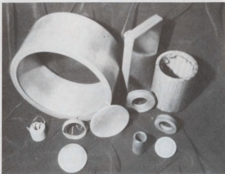
1. Piezoelectric ceramic materials are available in many shapes and sizes.
