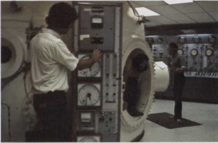
Hyperbaric research and training complex at Taylor Diving takes divers and equipment down to 2200 feet. Control console (background) indicates the intricate instrumentation that monitors the men's condition.
