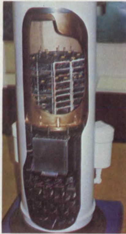
Electronic control unit for submerged well, by TRW, locks onto template, receives commands from surface via cable, decodes them and carries out the commands.
