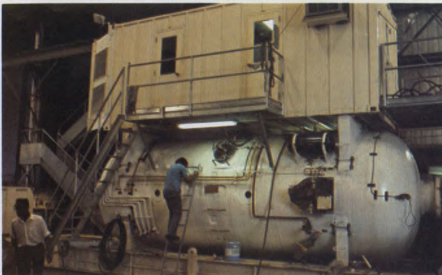
Environmental controls shack sits on top of Taylor's deck-mounted decompression chamber for divers. The men may stay in this chamber 30 days, leaving only for trips to the sea floor and back. The elaborate readouts in the control shack (above) are from transducers in the chamber that monitor the men.
