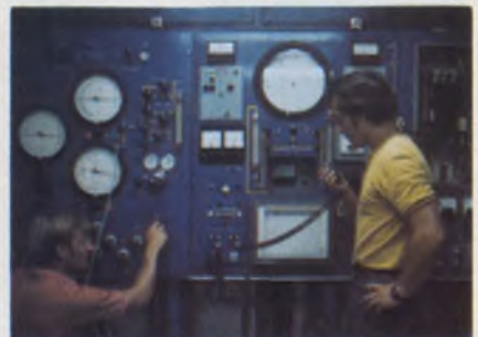
Environmental controls shack sits on top of Taylor's deck-mounted decompression chamber for divers. The men may stay in this chamber 30 days, leaving only for trips to the sea floor and back. The elaborate readouts in the control shack (above) are from transducers in the chamber that monitor the men.
