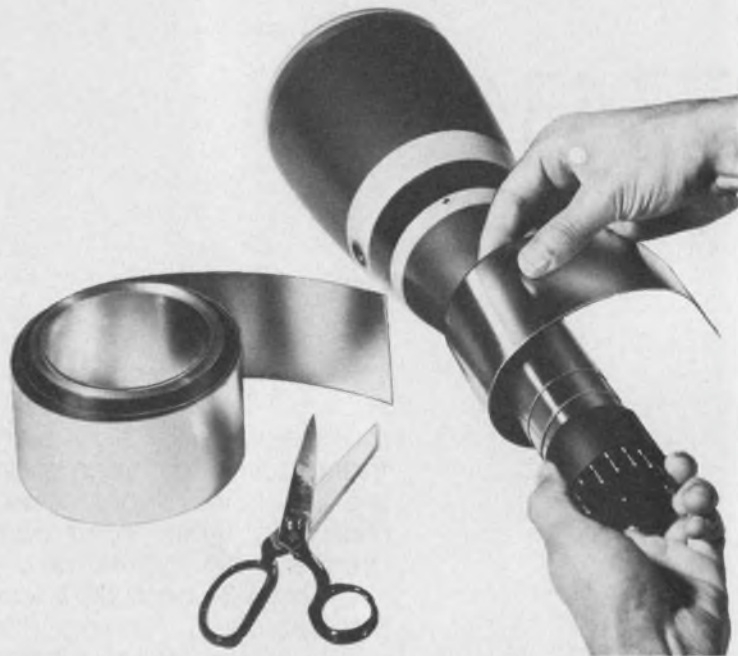
1. A pair of scissors and a roll or two of foil magnetic-alloy material are all you need to fabricate a practical magnetic shield.
