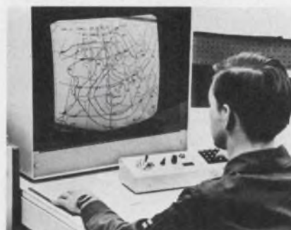
Weather conditions are observed on a CRT display of the Naval Environmental Display Station now under test at Monterey, Calif.
