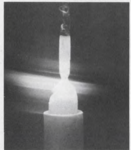
The top of the slug is melted by focused light. A seed crystal is then positioned above the molten cap (left), dipped into the cap (right) and then pulled slowly up to form a single crystal.
