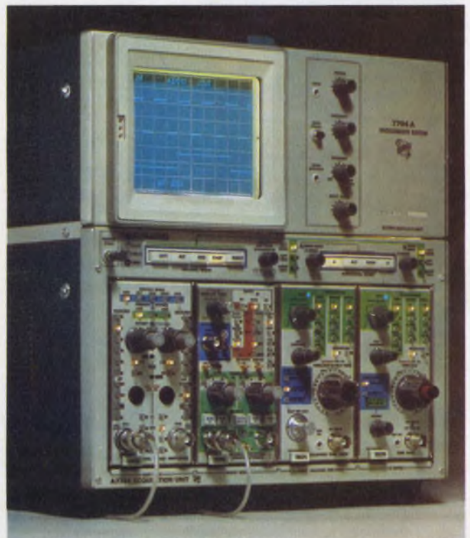
With the Tektronix 7D15—a universal counter/timer for the 7000-Series scope—you can display the count interval and a replica of the gating signal.
