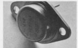
The first 3-amp positive IC regulator.
