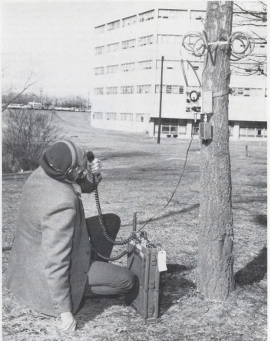
The tree above is radiating a signal at 10.803 MHz. Energy from the transmitter, operated by Kurt Ikrath, is coupled into the tree by means of a matching network in the box on the tree and the toroidal Hemac.
