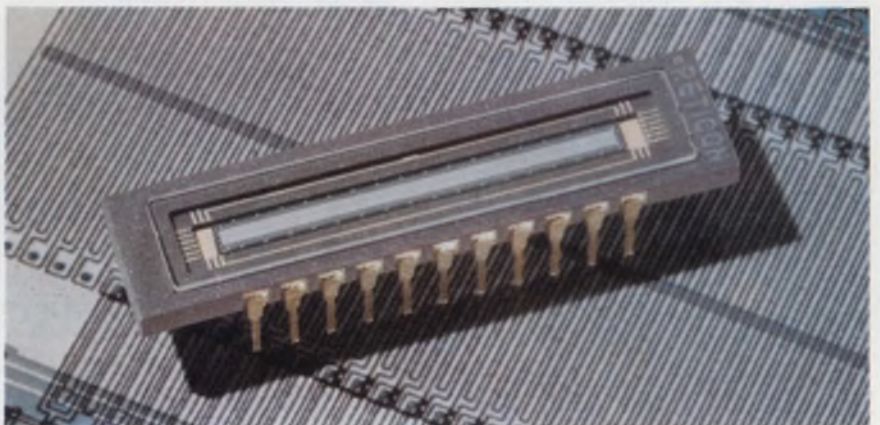
This linear 1024-element self-scanning array, by Reticon, uses gated diodes. The diodes are sampled by shift registers that open into common drains. Linear arrays like these have been used in line-scan and area-scan cameras.
