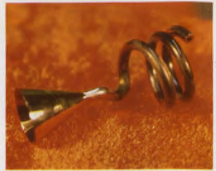
The flared input end of this channel multiplier, by Galileo Electro-optics, minimizes the device size.
