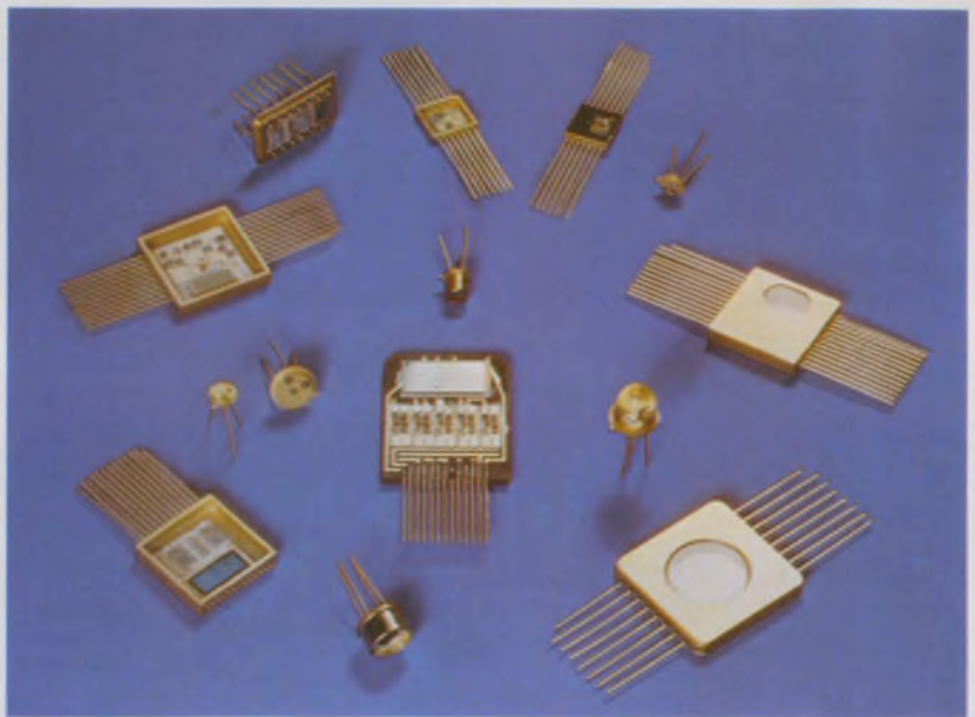
Operational amplifiers and video output amplifiers are combined, along with photosensors, in these hybrid packages by Meret. Designed for use in optical communications systems, they provide high sensitivity and power output.
