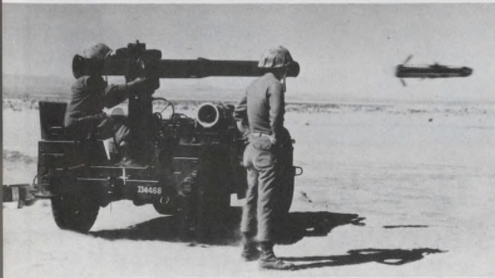
Antitank, wire-guided TOW missile, built by Hughes Aircraft, was launched by the Israelis from mobile tracked vehicles with great success.
