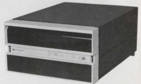
With this new mass memory, you can store or read a complete 250-line calculator program in about 2 seconds.
