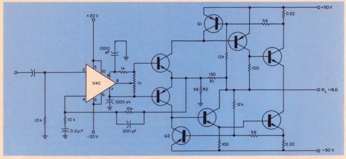
5. 75-W, 95-V-swing power amplifier uses two stages.
