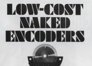
The Decitrak® naked encoder is specially designed for OEM applications . . . a stripped-down, low-cost incremental encoder easily integrated into systems designs. One part of the unit is a code disc easily mounted to your shaft; the other is an LED light source/photocell assembly ready for installation into your equipment. An economical, flexible solution to your systems design problems! Contact us today for a low, low quote and your free copy of our new applications brochure.
