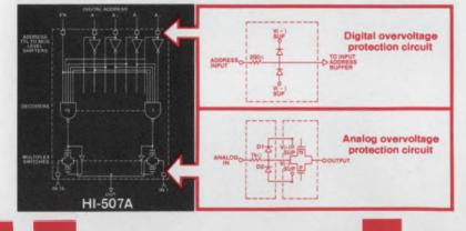
include data acquisition, telemetry systems, process control and general analog switching. The device is available in volume now for off-the-shelf delivery. For details see your Harris distributor or representative.
