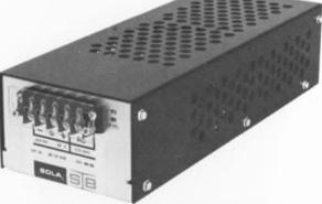
NEW MODULAR POWER SUPPLIES—CVDC □ Regulation—1% line, 4% to 10% load □ PARD -3% RMS □ Convection cooled □ Completely protected—short circuit proof □ Ferroresonant design, highly reliable □ Complete serviceability
