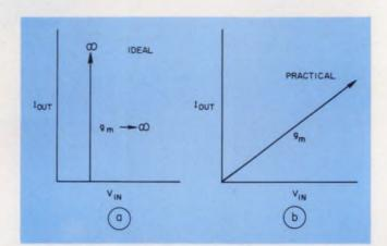
1. An ideal transconductance amplifier (a) has an infinite  $g_{\rm in}$  and, consequently, current. In practice, however, the current-vs-voltage curve is a linear function, with  $g_{\rm in}$  being the curve's slope (b).
