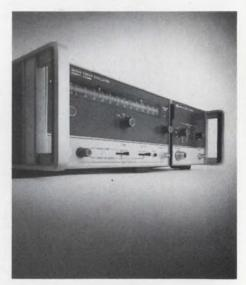
Easy to operate, HP's solid-state sweepers stress high performance from 3 MHz to 18 GHz.
