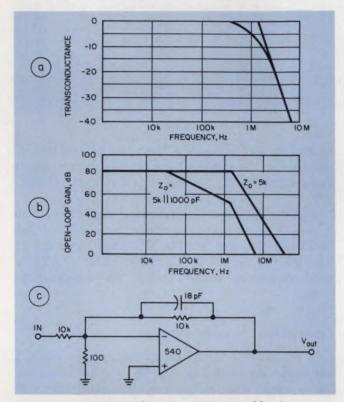
3. Constant transconductance over a wide frequency range is obtained when the load is resistive (a). Openloop voltage gain falls off faster when the load is capacitive (b). One way to compensate a power driver is to insert a lead network into the feedback loop (c).
