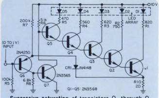
Successive saturation of transistors  $Q_1$  through  $Q_5$  give the LED display a bargraph appearance. Feedback through CR, helps linearize the apparent deflection as a function of input voltage.
