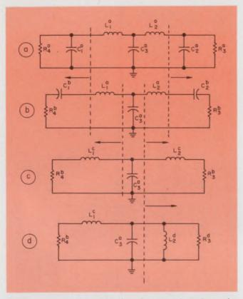
5. With resistors eliminated and source impedance included, the iteration begins with an arbitrary selection of  $L_a$ . The approximation of a lossless case is generally a close one for reasonable coil Qs.
