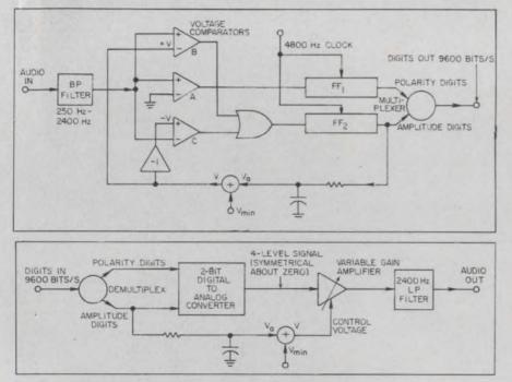
**Two-bit adaptive pulse-code modulation coder** (above) produces an output of 9600 b/s. At the receiving end the digits are demultiplexed by the two-bit decoder shown below.
