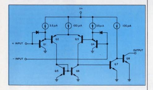
Unlike most comparators, the LM 139 can operate from a single power supply and still have an input common mode voltage range that includes ground. It is compatible with all forms of logic and has a power dissipation ranging from 570 mW to 900 mW, depending on the package.
