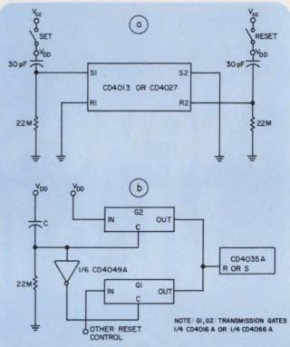
Simple RC network initializes CMOS memory element (a) because input-current requirements are low. The addition of a pair of transmission gates (b) provides turn-on initialization and system reset capability.
