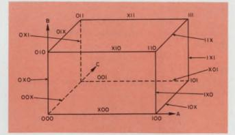
1. The universal cube for a three-variable Boolean function has 6 planes (2-cubes) and 12 edges (1-cube). In this topographical interpretation, vertices represent minterms; X's signify absence of a literal; and 1 denotes the variable and O, its complement. The literals in the are A, B, and C—in that order.
