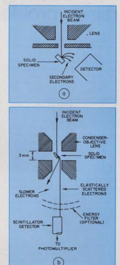
**Conventional electron microscopes** (a) use a long focal-length lens while IBM's new technique (b) allows the use of shorter lenses for higher resolution.
