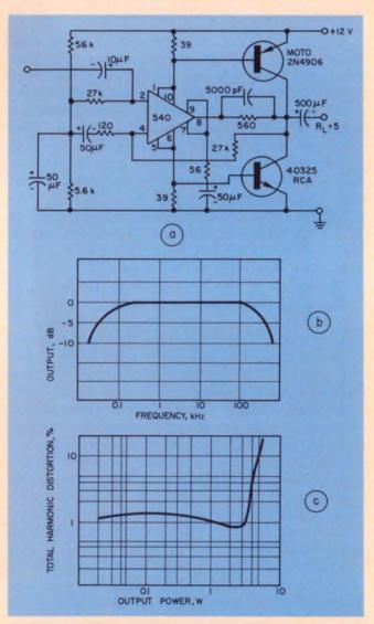
6. Power amplifier for a car radio (a) has a wide range of flat output vs frequency (at 0 dB, output is 1-V rms into  $5 \cdot \Omega$ ), as shown in b. The total harmonic distortion is relatively low over the range of useful power output (c).
