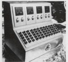
ISM Corp., 20 Sylvan, Woburn, Mass. 01801. (617) 935-6370. \$400. The Clockwatcher electronically totalizes the amount of time on a given project. Continuous monitoring of one to 15 stations is furnished via a visual digital display. Additional modules can increase capacity of the number of projects to be monitored. Operation of the Clockwatcher consists of pressing a button and setting the number of people working on a project. It even records overtime hours.
