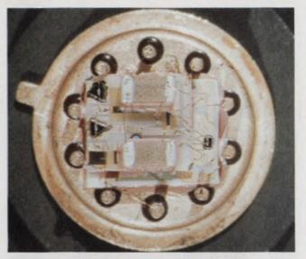
Halex's Model HX610 hybrid wideband amplifier delivers gain at frequencies beyond 100 MHz. When connected to a  $100 \cdot \Omega$  load the maximum output voltage at 100 MHz is 1.2 V pk-pk.
