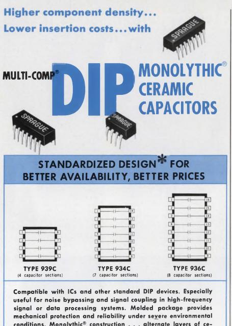
conditions. Monolythic<sup>®</sup> construction . . . alternate layers of ceramic dielectric material and metallic electrodes are fired into an almost indestructible homogeneous block. Standard ratings, 18 pF to 0.1  $\mu$ F @ 100 WVDC. Temperature range, -55C to +70C.
