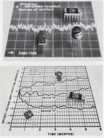
Precision Monolithics' OP-05A offers the best low noise (upper) and low drift (lower) specs for monolithic ICs.
