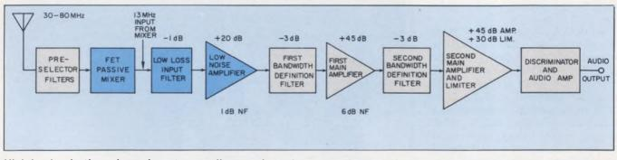
High-level rejection of nearby, strong adjacent channel signals was provided in the receiver, above, by use of new design techniques. The rf input stage was elimi-
