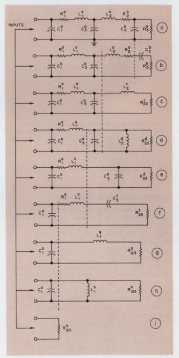
4. The general network reduces to a single, equivalent component by use of the relationships in the circular chart. For maximum power transfer, design the image input impedance— $R_{123}$ <sup>h</sup>—to equal the source impedance.
