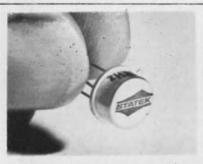
Rugged low cost quartz crystals in low profile TO-5 cans. 10 to 250 kHz frequency range.  $\pm 0.01\%$  calibration accuracy. Withstands 1000 Gs shock, 50 Gs vibration over 10 to 2000 Hz. Bypolar and MOS logic compatible. Price \$1.40 ea. in 10 K qtys. Circle number for literature. Statek Corp., 1233 Alvarez Ave., Orange, Ca. 92668. (714) 639-7810. INFORMATION RETRIEVAL NUMBER 156
