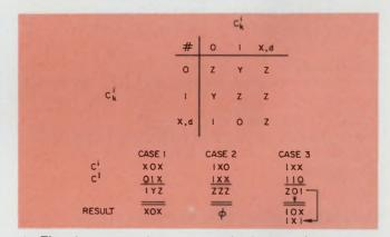
4. The sharp operation deletes all minterms from c that are common to c<sup>1</sup> and c<sup>3</sup>. Use the table for column-bycolumn comparison. Three courses of action are available; (1) copy c<sup>1</sup> if one or more Y's occur; (2) declare the result vacuous if all columns are Z; (3) copy c<sup>1</sup> for each occurrence of 1(0) and place the 1(0) in that column's position.
