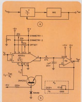
**True rms converter** increases its dynamic range by simultaneously squaring and square-rooting in the  $V_{in}^2/Z$  block (a). The actual circuit (b) requires only four trim adjustments and 13 components.
