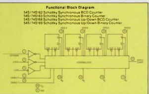
tended for use whenever bidirectional counting is required. The S162 and S163 are pin-compatible Schottky versions of the standard series 54/74 functions of the same number.
