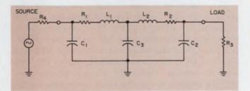
3. A general RLC network covers a variety of transfer functions often encountered. These include circuits for large-signal rf amplifiers.
