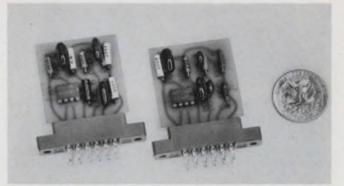
Active filters come in all shapes and sizes as demonstrated by the NAFI module made by Circuit Technology Corp. (left), the hand-held circuit card made by KTI (center) and the small plug-in circuit cards made by DeCoursey Engineering Labs (right).
