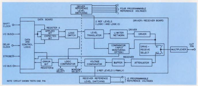
Driver receiver module handles a variety of logic levels. Each module can, on command, supply stimuli
