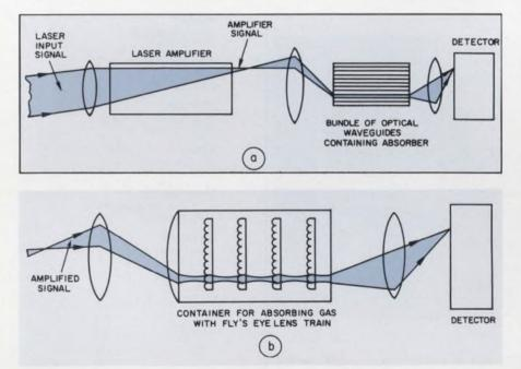
Wide-angle laser receivers with low noise and high sensitivity are seen as feasible with arrangements like those shown above. The absorbing element in both systems allows the signal to pass, yet blocks the noise.
