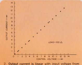
0 to 10 V. The circuit shown provides a scale factor of 0.96 mA/V.
