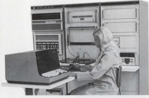
You don't need reference units because the 9560 system uses stored test patterns (truth tables). You can test at rates up to 22,000 patterns/second.
