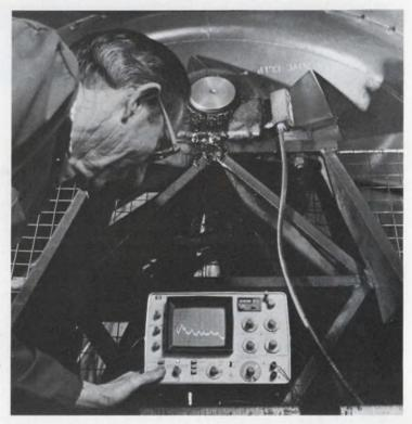
mode, from  $-150 \, dB$  to  $+30 \, dB$ . With digital storage, you can store a trace, then later recall and superimpose it on a subsequent trace for comparison. We even connected the discrete dots so the display is a sharp continuous line that looks like an analog display.
