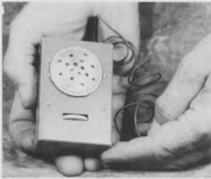
The Snooper , built by Gene Levette, is small enough (3-1/2-inches high) to be easily hidden. It transmits between 85 and 108 MHz for 1/4 mile. Its 9-V battery lasts 60 hours.
