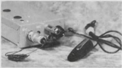
FM transmitter , high-powered and battery-operated, has a fountain-pen microphone, to be worn in the breast pocket. The antenna can be wrapped around the wearer's neck.
