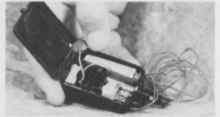
Small, wearable FM transmitter measures 1-1/4 by 2 by 1/2 inches. It operates on 0.5-W power for 1/4 mile. The battery lasts seven days. It's built by Gene Levette.
