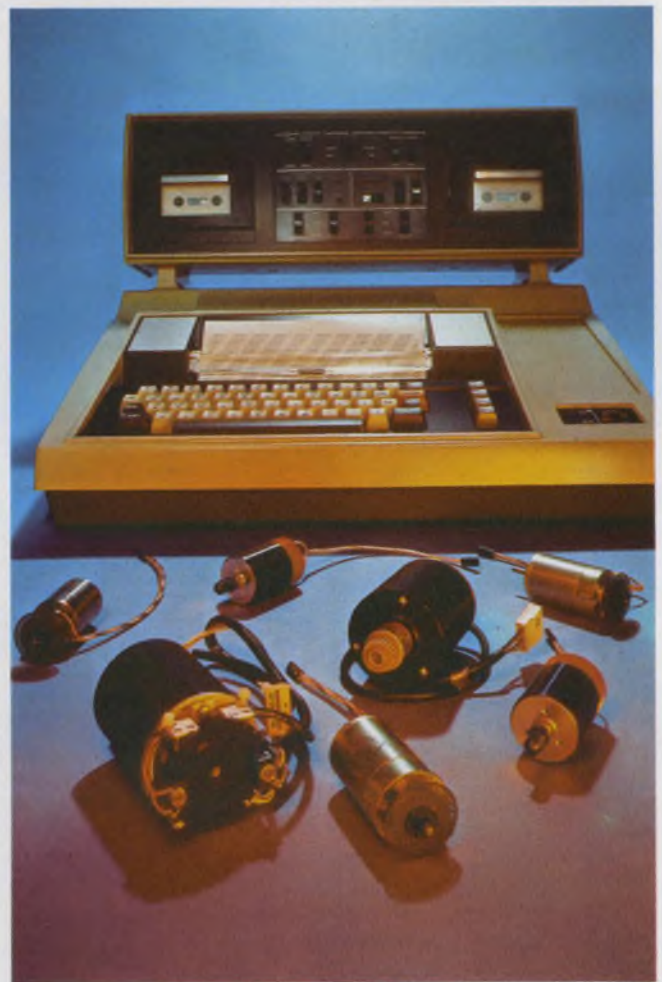
Though out of sight, electric motors are the workhorses of many computer peripherals. This Texas Instruments Silent 700 data terminal uses ten motors. Warner Electric Brake & Clutch stepping motors advance and return a thermal print head and advance the paper roll. Permanent-magnet dc torque motors provide mag-tape tension and fast forward and rewind, and servo-controlled capstan motors provide constant read/write tape speeds under phase-lock loop servo control.
