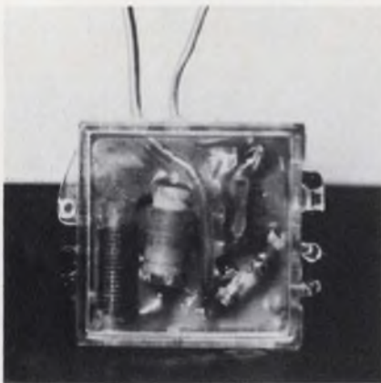
Tiny wiretap transmitter, built by Mickey Callahan, is about one inch square. Planted in a telephone, it transmits the conversation about six blocks at 88.5 MHz.
