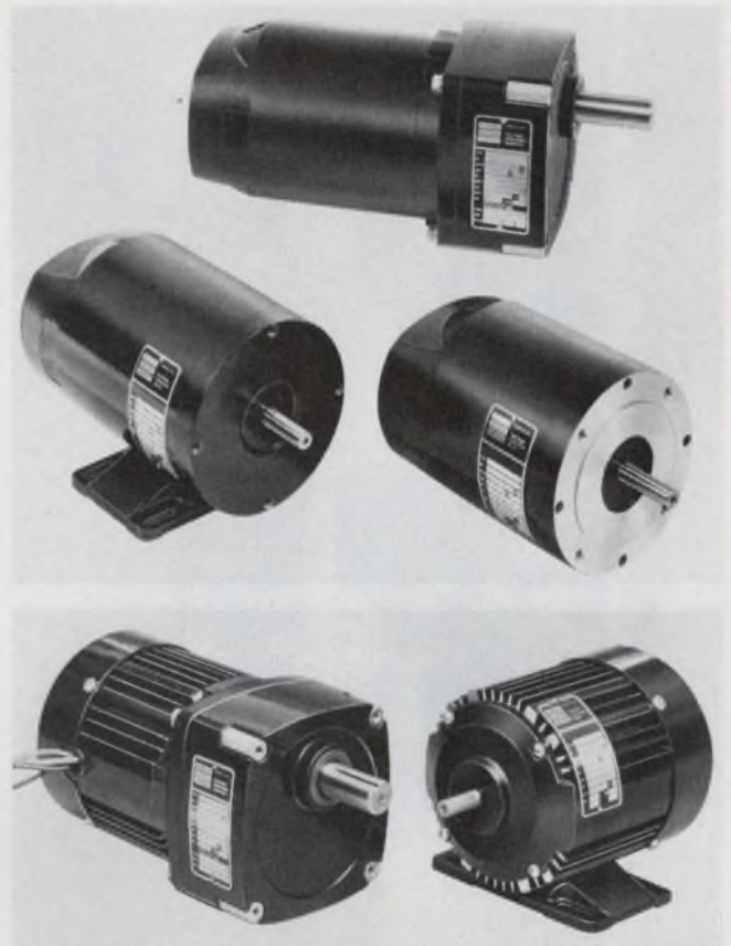
The external appearances of Bodine's permanent-magnet dc motors (top) and the more conventional ac induction motors (bottom), both in NEMA 42 sized frames, demonstrate the contrast in efficiency between the two motors. The induction motor needs fins and a totally enclosed fan to keep it cool.
