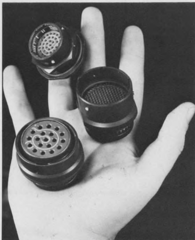
1. If you're using circular multipin connectors, such as these MIL-C-81511 versions, you must select a size that can handle your maximum load current without exceeding the temperature rating.
