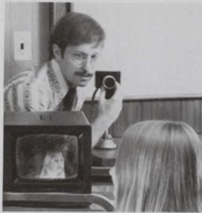
First charge-coupled television camera produced by Fairchild.
