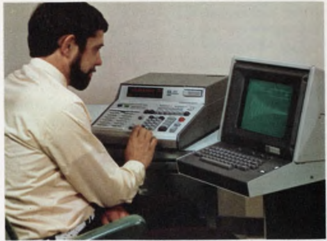
Model 31 programmable scientific desk-top calculator from Tektronix is operated with the company's 40101 graphic display terminal (Session 27).
