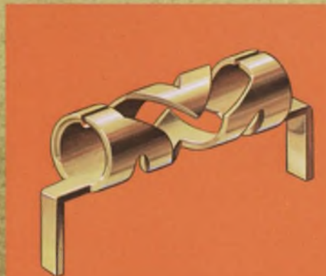
Dual chevron-shaped springs provide positive contact and grip between receptacle and pin, and minimize overall length and diameter of mated contacts.
