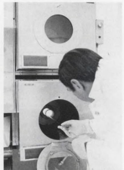
Specialized ICs are a big R&D effort at Fort Monmouth. The technician here is putting a tray of MOS IC wafers into a diffusion furnace.
