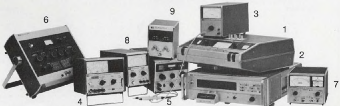
No. 1: 4342A Q Meter. No. 2: 4270A Automatic Capacitance Bridge. No. 3: 4328A Milliohmeter. No. 4: 4329A High Resistance Meter. No. 5: 4260A Universal Bridge. No. 6: 4265A Universal Bridge. No. 7: 4350A High-Capacitance Meter. No. 8: 4332A LCR Meter. No. 9: 4050A Analog Comparator.
