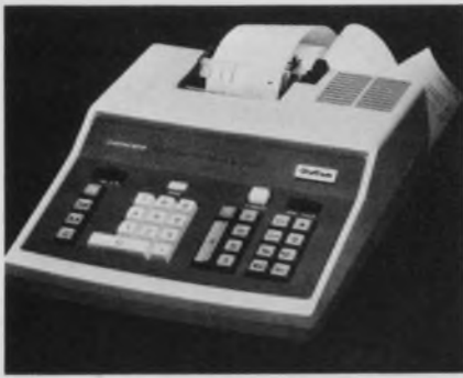
Electronic calculators with printout, like this Unicom 500P, use buffers between the calculator chip and printer.
