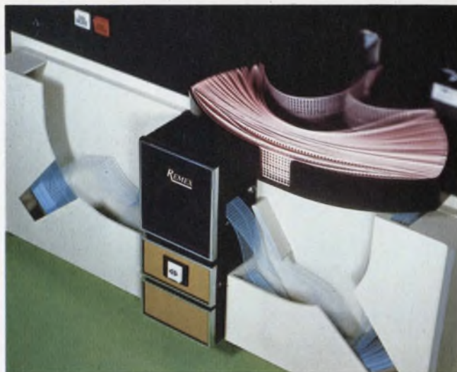
With a fully asynchronous 300-cps reader and a fully asynchronous 75-cps paper-tape punch in the same box, the RAF 6375 from Remex hits the major needs of the industrial-control market.
