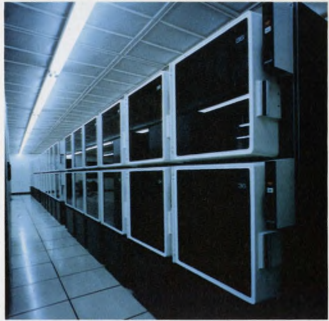
Ampex's terabit memory system has a capacity of 3 \times 10^{12} bits and an access time of 10 s.
