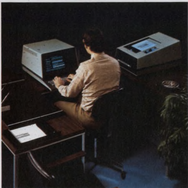
Tektronix' 4023 Computer Display Terminal and 4632 Hard Copy Unit provide a low-cost terminal system with upper and lower-case characters and format control.
