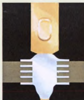
Contact is flow soldered in place, producing uniform fillet with full solder, top to bottom, and clean, solder-free posts.
