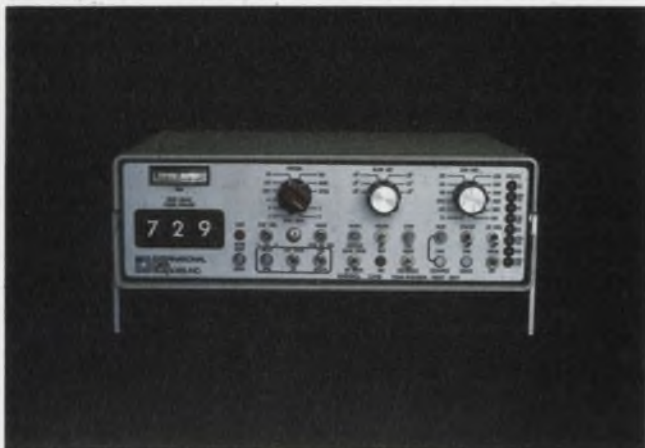
You can test digital data communication systems with International Data Sciences' Model 1310. The unit generates pseudorandom start-stop characters.
