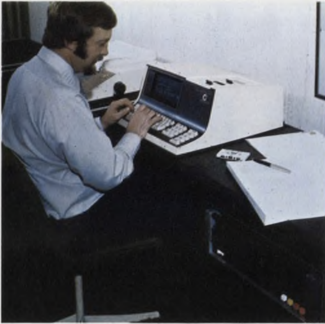
Datapoint's 2200 intelligent terminal offers an alpha-numeric keyboard for data entry, a CRT for data display and two digital cassette recorders for bulk data storage. The 2200 is programmable and comes with up to 16-k, eight-bit words of storage.
