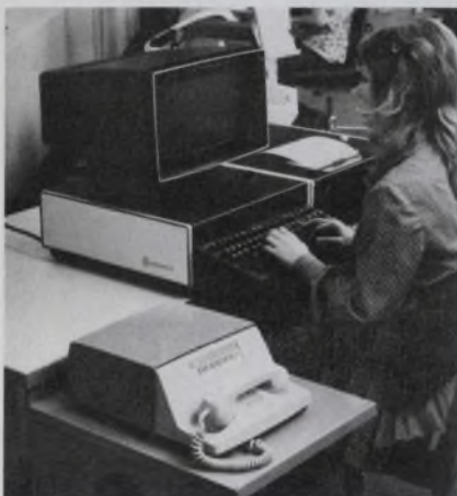
AT&T's new data terminal features a combination high-speed printer and cathode-ray-tube display.
