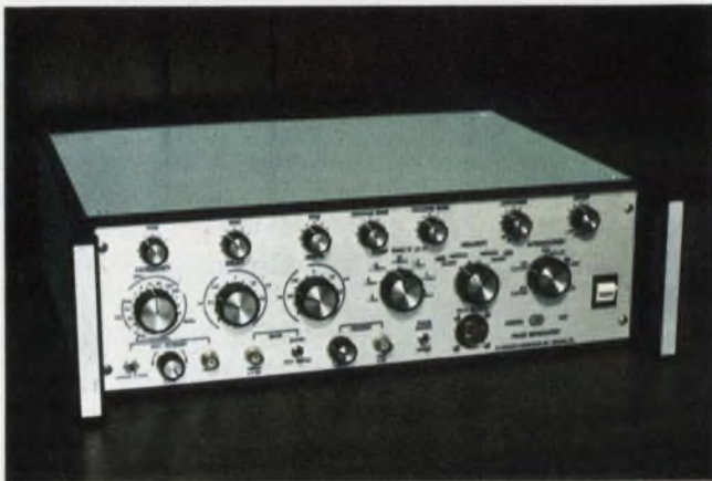
E-H Research Laboratories' Model 137 features a rep rate of 100 MHz, variable rise and fall ramps from 0.5 ns/V to 40 \mu s/V and variable baseline offset to \pm 5 V. Delay and width are also variable.
