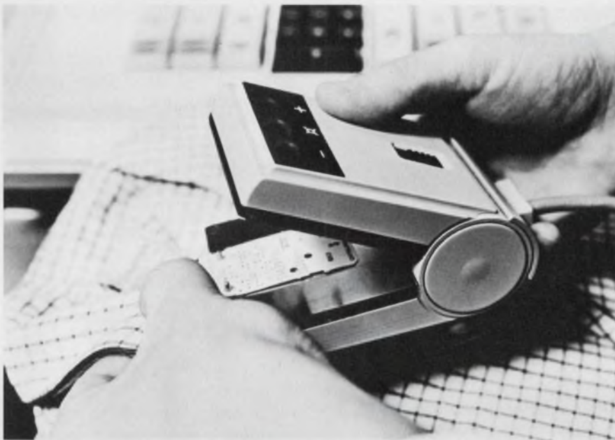
This merchandise ticket reader—the Friden Model 705, built by the Singer Co.—automatically reads and records coded information.
