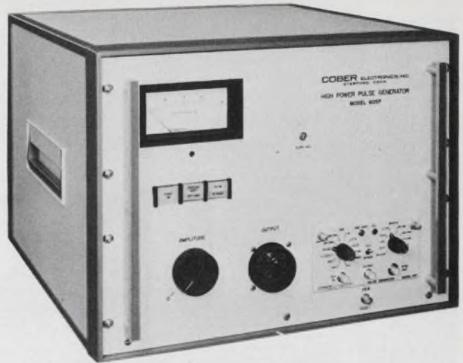
A peak of 24 kW is obtainable from the 605P, Cober Electronics' high-power pulse generator. Minimum width of the 11-A, 2.2-kV pulse is 50 ns.
