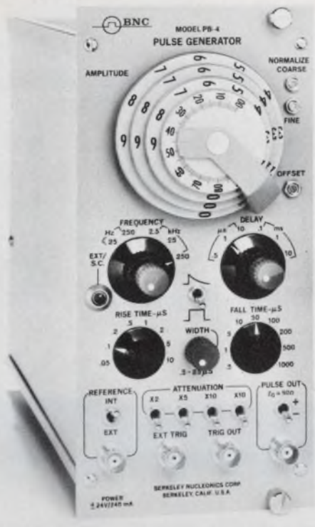
Berkeley Nucleonics' PB-4 is a precision pulser that provides a highly linear tail or flat-top pulse.
