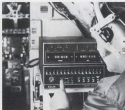
Ruggednova, shown above, is aboard a Sabreliner jet performing data acquisition and navigation functions for atmospheric research.
