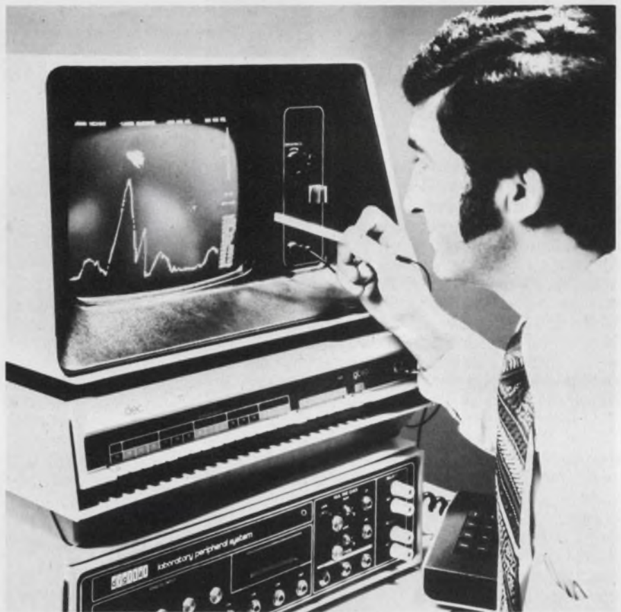
Intelligent terminals, such as this one from Digital Equipment Corp., contain a minicomputer that can be used to preprocess information for the CPU.
