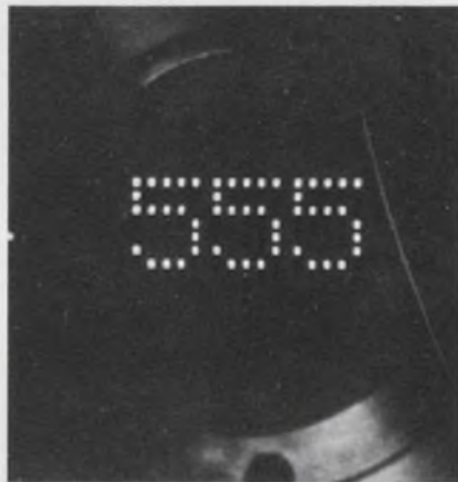
Incandescent display developed by IBM is brighter than LEDs at the same power consumption.
