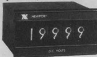
SERIES 2000B DPM: ±19,999 counts • DC voltage and current models 30 rdgs/sec • 2½"H x 4½"W x 5"D. • 0.01% accuracy • BIG-BCD output
