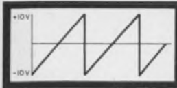
Sawtooth waveform ERMS = 5.77 Volts; 17.4 dBm
