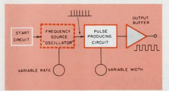
oscillator. These pulses then trigger a monostable multivibrator with adjustable time constant which determines the output pulse width. Output buffer provides additional amplification.
