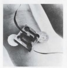
As positive or negative strain is applied across the strain axis of the gage, the capacitor plates either expand apart or contract together. Although the plates are initially in a state of mild compression, they can still compress further together due to the crushability of the Mica.
