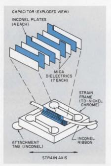
The gage has a mass of 1.0 gram and a nominal capacitance of about 10 pF.
