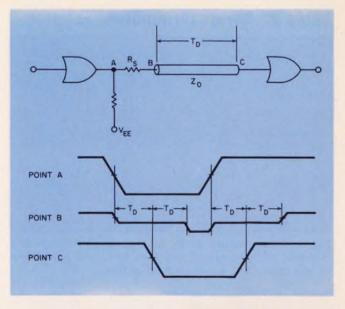
4. Series-terminated lines don't need the extra power supply. But you can't have distributed fanouts because of the half-voltage waveform on the line (waveform B).
