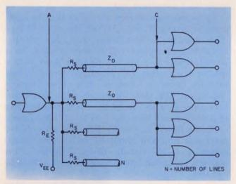
5. With N lines, N loads are obtained on a series-terminated line. Resistor  $R_{\rm E}$  must be less than a maximum value fixed by the number of lines and  $Z_0$  to prevent the output transistor from turning off during switching.
