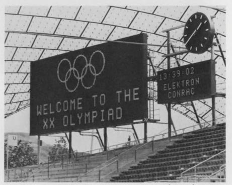
**Two giant, computer-controlled displays,** designed by Conrac Corp., have been installed in the Olympic Stadium in Munich, the principal site of the Summer Olympic Games. These boards use up to 1.26 MW for operation.
