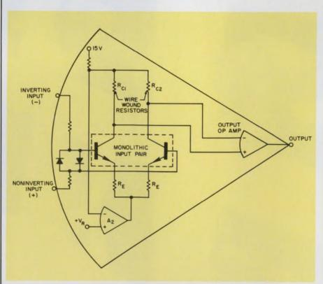
Modular op amp exhibits improved stability with time and temperature when an IC op amp and matched, wire wound resistors are used in the monolithic input-pair stage. Another IC op amp is used in the output stage.
