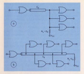
3. Parallel-terminated lines can have lumped (a) or distributed (b), fanouts. A termination voltage,  $V_{\rm TT}$ , is required to prevent excessive termination-resistor power.
