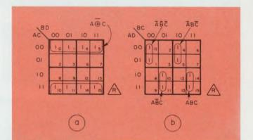
5. To detect EXCLUSIVE-ORs that don't cross boundaries, the map of Fig. 4 is redrawn by combining row and column variables. A is combined with C in "a" and with D in "b."
