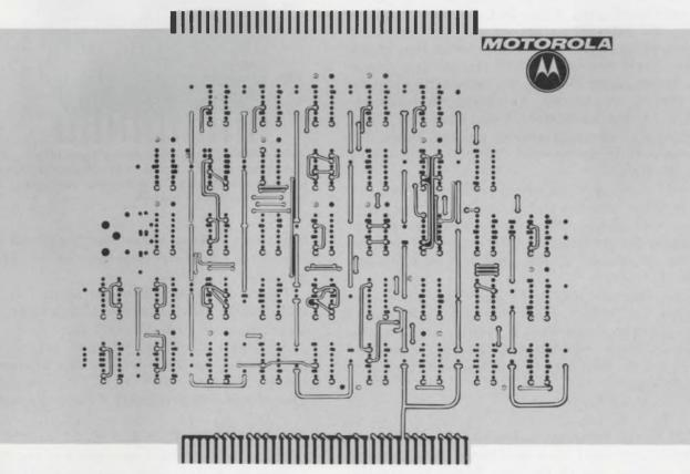
1. A MECL 10,000 PC board with a ground plane. The board provides a constant characteristic impedance and low inductance path for ground currents. The ground plane also serves to maintain a noise-free voltage plane for the  $V_{\rm CC}$  supply. About 30 to 40% of the ground plane is removed for signal interconnections.
