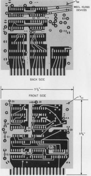
2. You don't always need the ground plane, as in this high-speed counter layout. The capacitors provide low frequency bypassing. Signal lines are short, and no transmission lines are used.
