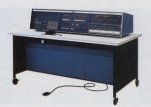
The Model 4400, which Datatron says was the first system to use force/monitor circuitry at each device pin.
