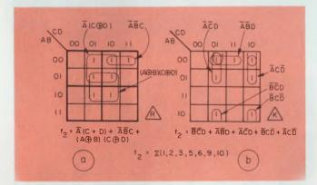
3. Functions containing mixed terms are easily handled by the Ring map (a). The standard Karnaugh procedure is shown in (b).
