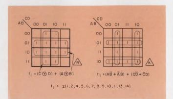
2. **EXCLUSIVE-OR functions** contained in  $f_1$  are spotted immediately on the Ring map, but the Boolean equation for  $f_1$  that is derived from the Karnaugh map must be manipulated to minimize the function.
