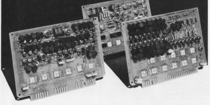
Kearfott can solve your synchro-to-digital and digital-to-synchro conversion problems with three production model solid state converters. All three meet MIL-E-5400.\* TRIGAC I—A low cost synchro to digital converter, accurate to 12 minutes.
