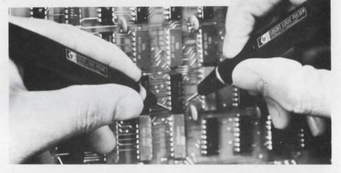
the logic clip to flip-flops, counters, decoders, shift registers, and other MSI chips; then monitor exact operation 14 or 16 pins at a time with the pulser providing clock, reset, clear or transfer pulses.
