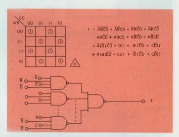
6. Karnaugh reduction in this example results in a circuit that requires five DIPs and 32 inputs. Contrast this with the Ring-map reduction in Fig. 7.
