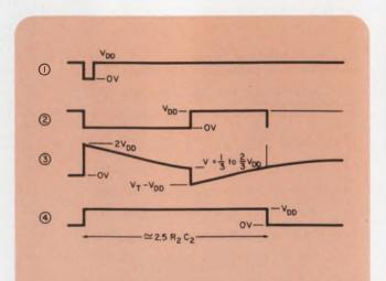
2. Waveforms show the output pulse triggered by a ZERO at the set input.
