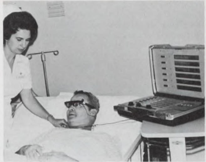
The sight switch, developed originally for the U.S. space program, is being incorporated in control systems for fully paralyzed patients. (Session 2G.3).
