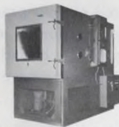
TenneyZphere For simulation of temperature, humidity, vacuum.
