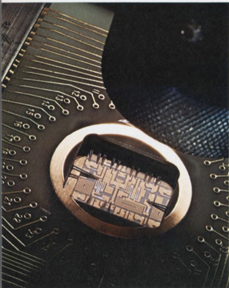
At Motorola Semiconductor, a two-stage complementary symmetry line extender is trimmed on a laser system. The thin-film hybrid includes inductors (square loops).
