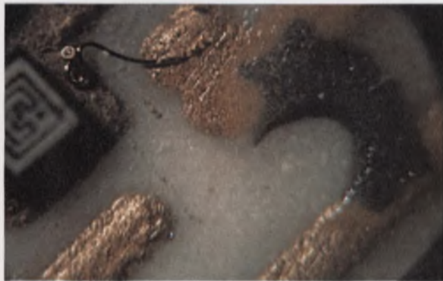
Trimming the S.S. White way means Airbrasive equipment (left). Available nozzle openings are as small as 5 mils, and the shape can be either round or rectangular. Functional trimming is also possible (above), but generally this requires a coating over the active components for protection. System prices start at $6000.
