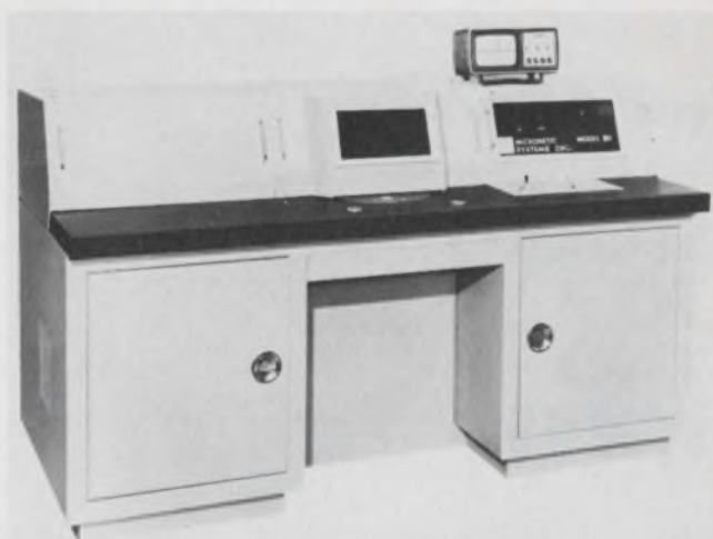
Micronetic's model 80 lists 15,000 trims per hour to 0.1% accuracies. At a base price of $59,000, the unit uses a Q-switched YAG with rep rates up to 10 pps.
