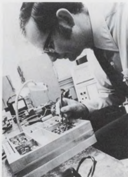
Prototype of mobile telephone unit at Bell Laboratories will be used in a new high-capacity, low-power mobile communication system.
