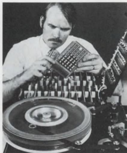
A low-power digital circuit card of the data logging system is checked by James Nick of Honeywell.
