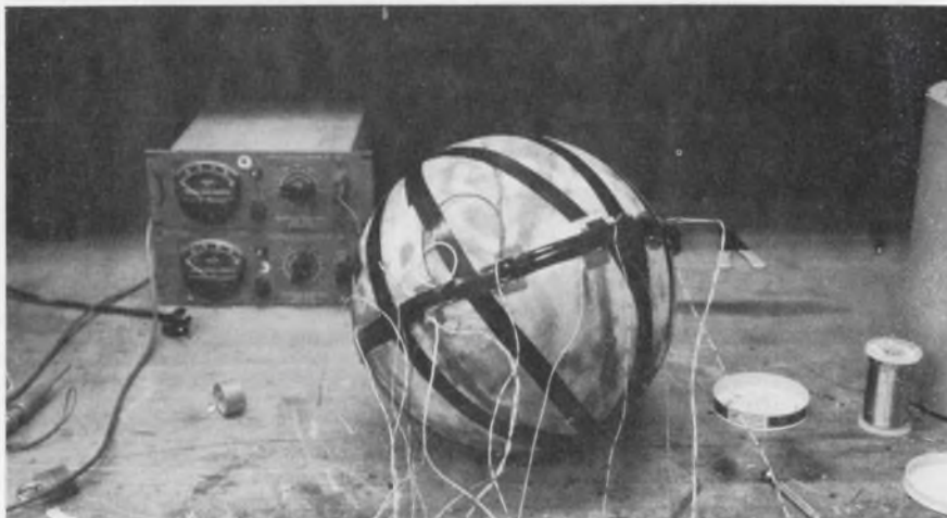
Both temperature-control and data-readout thermal sensors are inserted in the insulating foam inside both the 4-inch and the 11.5-inch ovens. Connections to the sensors and oven heaters are brought out.
