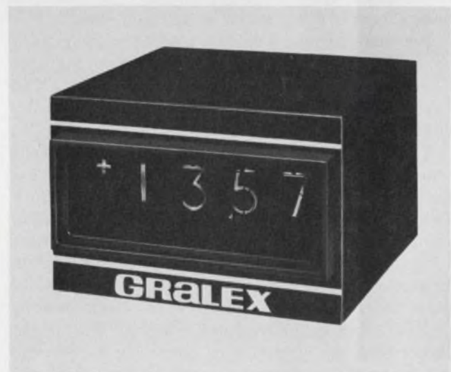
Simple behind-the-panel mounting is offered with the series 35 3-1/2-digit meters from Gralex Industries. Features include 5/8-in.-high display characters and a rear-panel control that permits the scaling factor to be linearly varied for matching to transducer inputs.
