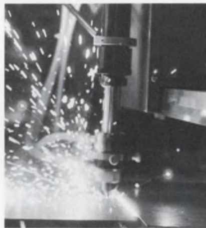
Cw gas laser slices through a 0.39-inch-thick titanium sheet at 100 inches per minute. Called the Laser-Matic, the unit is made by the Liquid Carbonic Corp.
