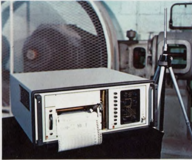
General Radio's GR1523 Level Recorder operates fully automatically here, recording a one-third octave analysis of the noise generated by the nearby compressor.
