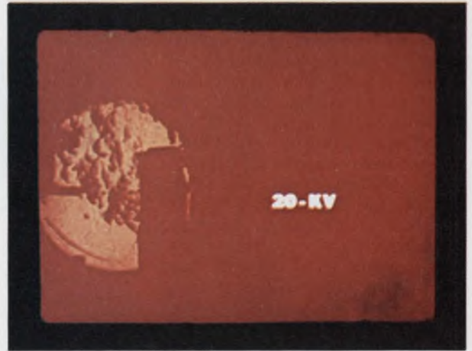
namics, a 1100-F copper plate has minimum heat transfer with no field. At the right, the turbulence of a 20-kV field lowers temperature 300 F.
