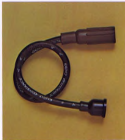
The resistive path in most approved ignition wire cables is made of a glass or linen fiber—impregnated with a coating of graphite.
