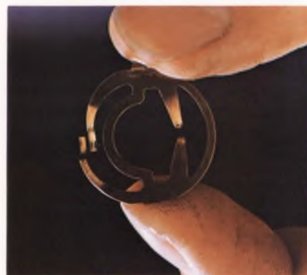
The fine copper springs used in contacting resistors can be coated with conductive/lubricating coatings. This provides for longer life before high electronic noise levels are reached.
