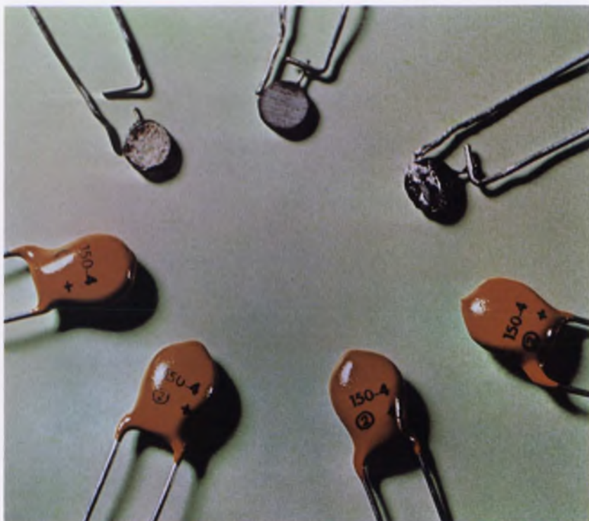
These tantalum capacitors make use of both silver and graphite coatings. Their small size and high capacity make them of special use.
