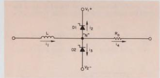
2. Current summation at node N is the basis of converter operation. With the output open-circuited, the instantaneous voltage at "N" is either V<sub>1+</sub> or V<sub>2-</sub>.
