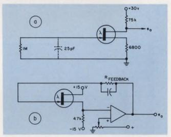
9. The basic circuit of a photo FET (a) shows the gate-todrain capacitance, which limits frequency response. The effect is overcome by using an operational amplifier (b).
