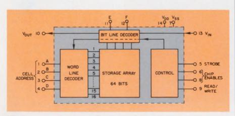
Ultra-low-power dissipation CMOS RAM has decoding and control circuits on one chip. The memory is organized as 64 words by 1 bit.
