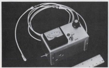
An MEM 520 p-channel MOS transistor is the radiation sensor in this model of the Mosimeter. Three ranges are available: 20, 100 and 500 rads. Up to 100 feet of coax can be used between the sensor and the meter box.
