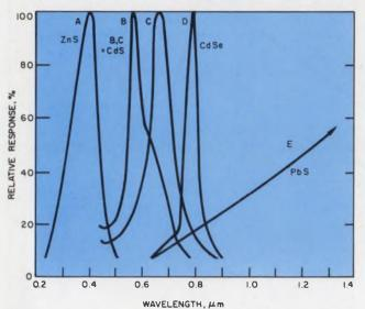
2. The response of cadimum sulfide (B,C) and cadimum selenide (D) photoconductive cells is primarily in the visible region, while zinc sulfide (A) responds in the ultraviolet. Lead sulfide (E) is useful in the infrared.
