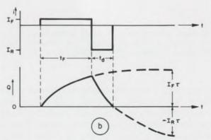
B. Constant current (top) and charge waveforms show that the time,  $t_{\rm d}$ , to remove the stored charge from a pulse snap diode is dependent on the reverse current,  $l_{\rm R}$ , through the diode.
