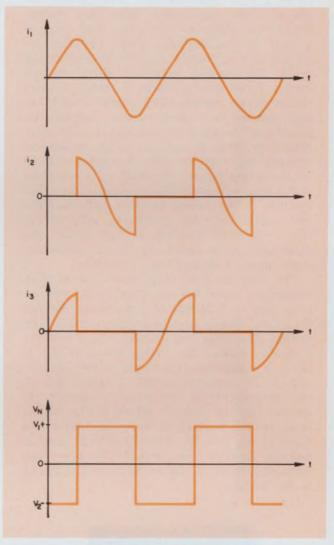
3. Waveforms for converter of Fig. 1 show that the area under the forward-current curve for the diodes is the same as the area under the reverse-current curve.
