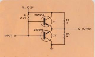
**Low-value equal resistors** across the output of this complementary emitter driver improve its noise immunity by making it less sensitive to load conditions. Crosstalk is also reduced.
