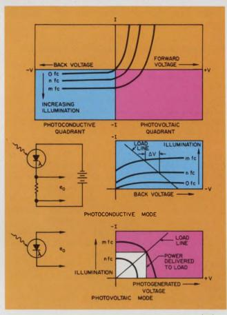
12. Photovoltaic cells, as well as any pn junction device, can be operated either in the photoconductive mode or the photovoltaic mode. The top curves (A) are shown with quadrants as normally drawn. In B and C the quadrants have been reoriented, for simplicity.
