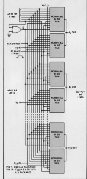
It's simple and practical using Motorola's extremely low power Mc-MOS. The 128-word by 24-bit Static Random Access Memory shown is just one of the many medium speed, micropower organizations possible with the flexible design of the latest addition to this rapidly expanding complementary MOS line, the MCM14505L 64-bit RAM.
