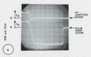
A. **Difference in switching characteristics** of pulse snap diodes and pn junction diodes are obvious from these traces of the reverse-current turn-off characteristic of each.
