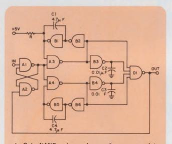
1. Only NAND gates and capacitors are used to build this variable-delay circuit. Capacitors  $C_1$  and  $C_4$  control timing. Resistor R is optional if additional fine control is needed.
