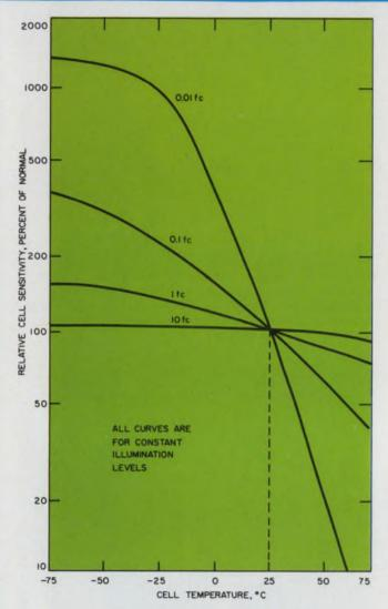
15. Temperature changes affect photoconductive cell current and sensitivity. These curves show typical variations for a cell under differing levels of illumination.
