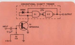
Vary the threshold of your Schmitt trigger with the addition of just a single transistor. The "modified" circuit is sensitive to 50-mV triggering levels at frequencies of up to 20 MHz.
