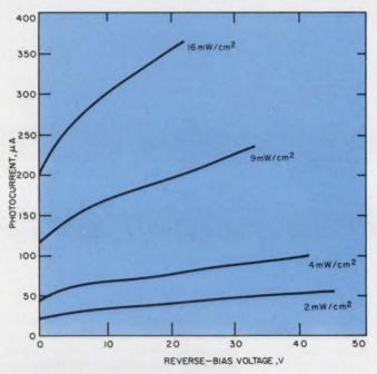
5. Increases in both illumination and back-bias voltage of a silicon photodiode raise the output current levels. In the example here, the illumination on the junction of a Texas Instruments 1N275 lies in a band between 0.7 and 1.1  $\mu$ m, at a cell temperature of 25°C.
