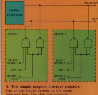
interrupt line. The skip line provides a means for device identification.
