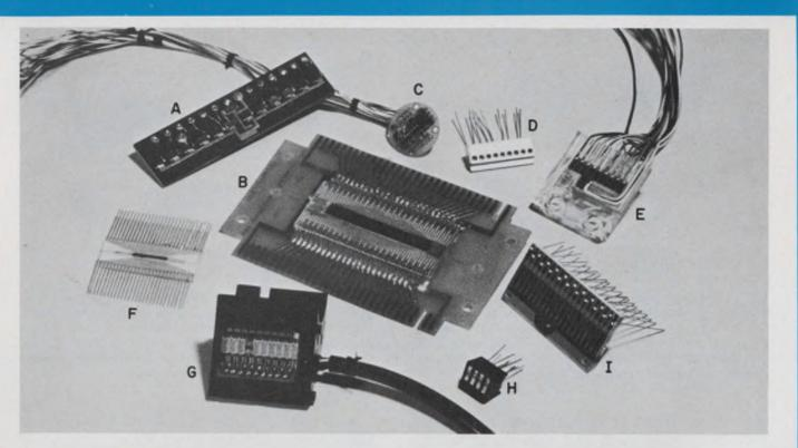
17. Photodiodes, phototransistors and photoconductive cells are used in optoelectronic arrays. Examples of silicon photovoltaic arrays are found in a card reader (A), optical decoder (C) and punched-tape reader (G) by Sensor Technology, and a tape reader (E) by Solar Systems. The Sensor Technology reader has hybrid amplifiers to mate the cell outputs directly with TTL
