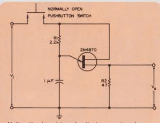
Unijunction-transistor circuit stops contact bounce by supplying a pulse with a 200-ns rise-time. Resistor  $R_1$  permits the UJT to fire only once by overriding the device's valley current. ess cos
