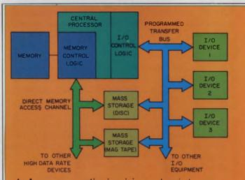
4. A common practice in minicomputers is to use separate buses for programmed transfer and direct memory access (DMA). DMA requires more complex hardware but handles higher data rates.
