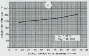
C. Transition time vs stored charge curve for an SV110 pulse snap diode shows the increase in transition time for additional amounts of stored charge. Stored charge is a function of time and  $I_{\rm F}$ .
