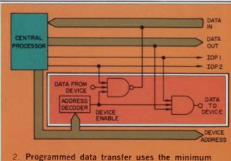
number of interface components. These are an address decoder, a bus driver and a receiver.
