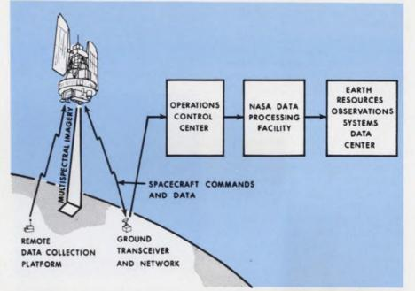
The ERTS satellite will send data it collects plus that from ground-based platforms to Goddard's ground stations, then to a control facility, to data processing, and on to the data supply center in Sioux Falls, S. D.
