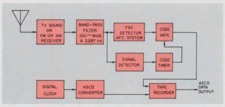
An aural system for identification of ads, by Audicom, uses frequency-shiftkeyed audio signals that are buried in the ad by being sent with a  $\pm 35$ -Hz bandwidth and at a level of 50 dB below 100% modulation. A 100-Hz notch filter, with a 2877-Hz center frequency, is used to insert or to retrieve the signals. The monitored output is operative only when the presence of the frequency-shifted signal is noted by the signal detector.
