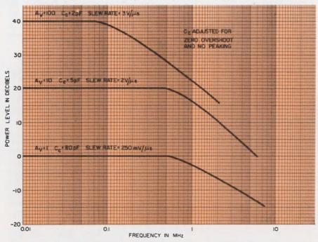
The  $\mu$ A791 op amp has a flat response to nearly 1 MHz, for unity voltage gains (lower curve). Responses for higher gains are also shown.
