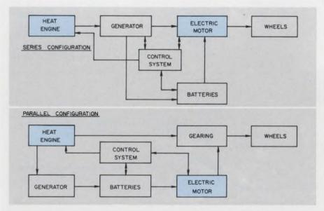
Hybrid electric motors can be designed in either series or parallel configurations. While the series configuration is more flexible and can be produced at a lower cost, the parallel configuration gives lower exhaust emissions by 10% to 20% and is therefore the choice of Aerospace Corp. designers. due to greater efficiency. This configuration is 10% to 20% more efficient than the series configuration. The main advantages of the series configuration are simplicity, flexibility and lower cost."
