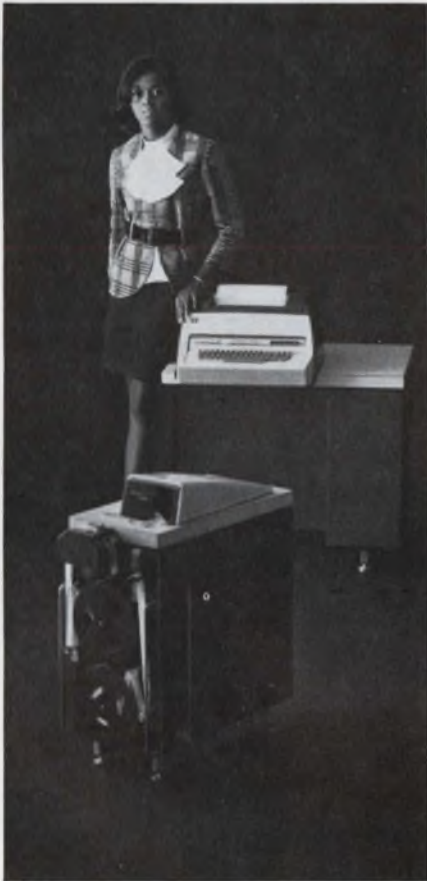
model 37 series: One of the most versatile heavy-duty terminal lines going. Generates all 128 characters of ASCII. Operates at 150 wpm. Prints in upper and lower case.
