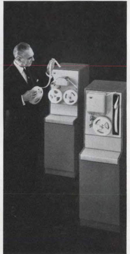
Telespeed™ equipment: A line of high-speed tape-to-tape terminals capable of sending and receiving at speeds of 750, 1050 (shown above), or 1200 words per minute.
