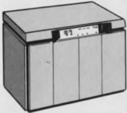
CM 1700 Large Core Store — An advanced high-speed random access mass memory providing up to 20 million bits
