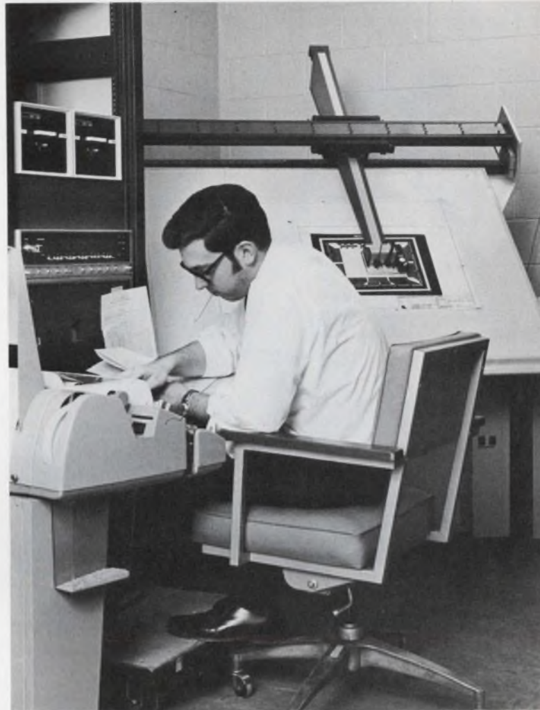
The Designer II, an automated drafting system made by Computervision Corp., Burlington, Mass., enables engineers to sketch several complex electronic designs per day. Once a final design is selected the system, based on a Nova minicomputer, prints out final drawings to mil spec standards. Layouts, assembly drawings, bills of material and numerical-control manufacturing tapes are easily extracted from the new system.
