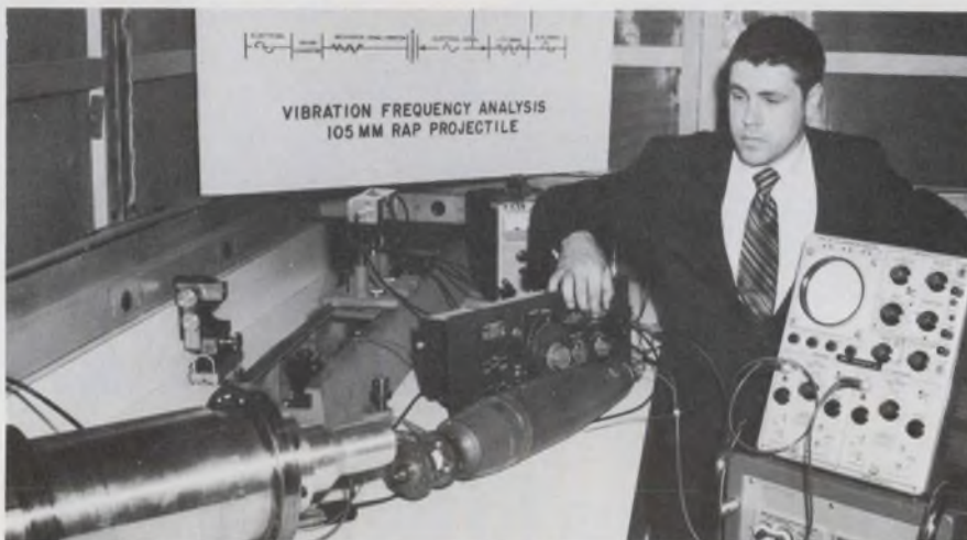
Electro-optical transmitter, examined here by its inventor, John Bera of Picatinny Arsenal, sends vibration data on 105-mm rotating projectile.
