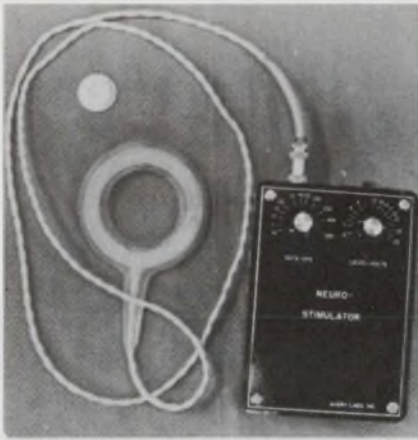
Experimental neuro-stimulator consists of a transmitter with a coiled loop antenna. The antenna is placed over an implanted receiver.
