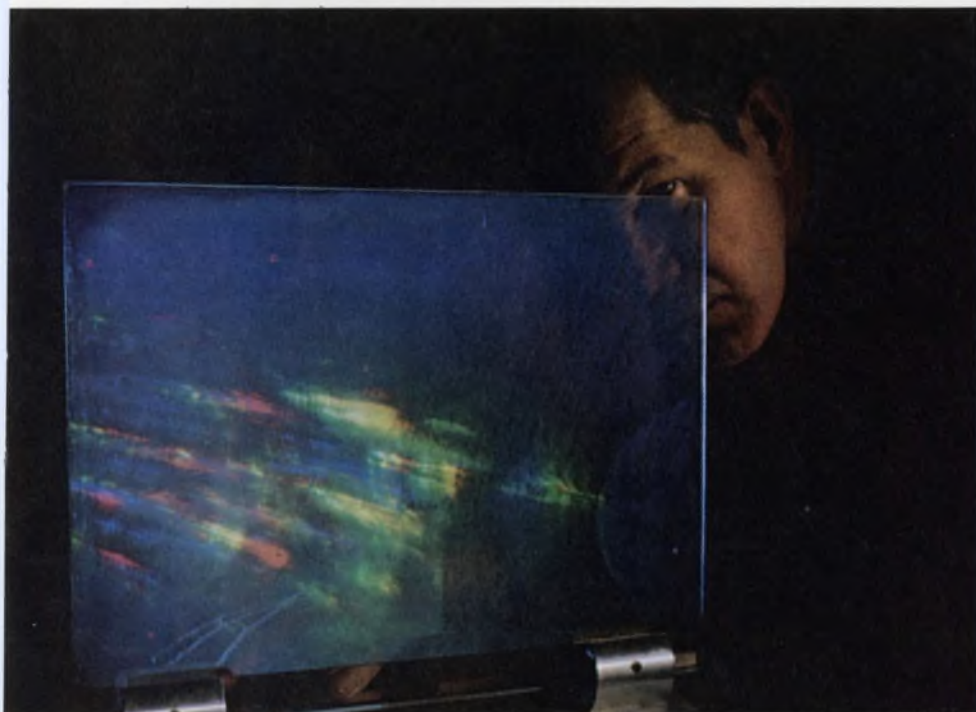
A composition of glass objects and spheres, this American Optical hologram, created by Harriet Casdin Silver and made by Larry Okonski, is viewed with a mercury arc. Diffraction of the white light creates the many colors.
