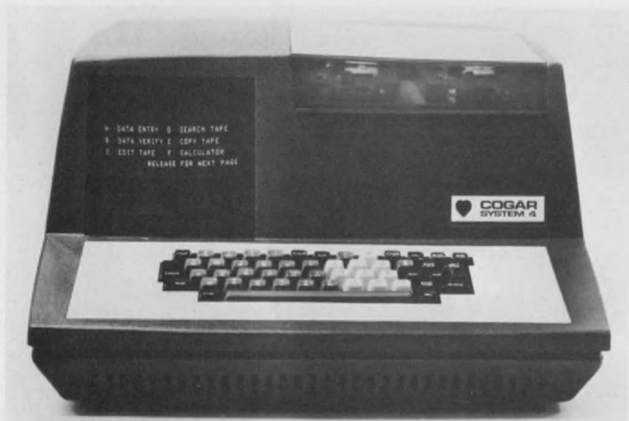
Using a typewriter keyboard the Cogar 4 records data on tape cartridges.
