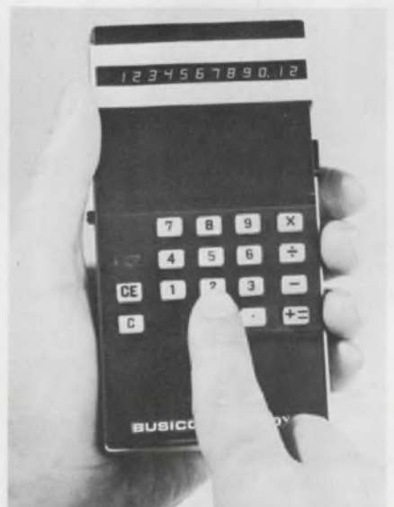
Battery operated pocket calculator will have a light-emitting diode display.
