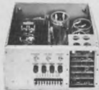
Multi-Output Supply Independent regulator for each output. Sequencing and control circuits on plug-in cards.
