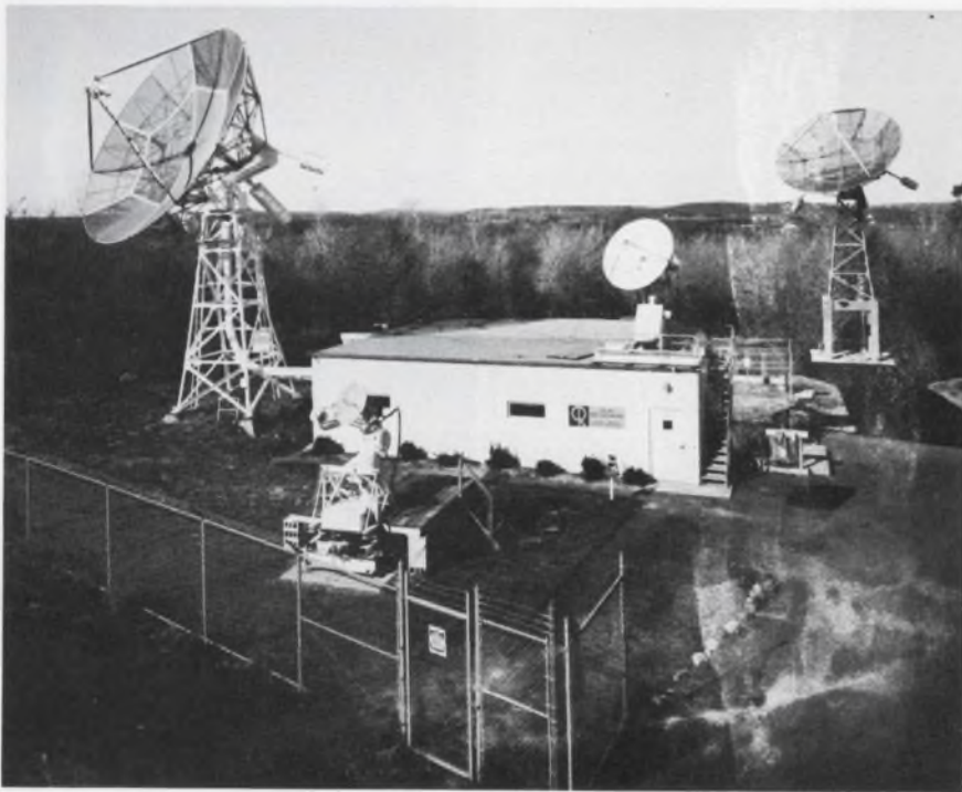
Solar activity is monitored in different frequencies by these five antennas at the Air Force Cambridge Research Laboratories' solar radio observatory near Ipswich, Mass. From left to right: the 28-foot antenna receives solar emissions at 606 MHz and 1415 MHz; the 1-foot antenna in the foreground attached to its 3-foot companion on the right receives at 35,000 MHz; the 3-foot dish is tuned in at 15,400 MHz; the 8-foot antenna on the observatory roof receives at 2695 MHz, 8800 MHz and 4995 MHz; the 28-foot dish at the right of the building receives at 245 MHz.
