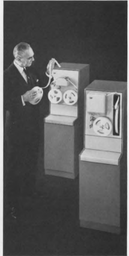
Telespeed™ equipment: A line of high-speed tape-to-tape terminals capable of sending and receiving at speeds of 750, 1050 (shown above), or 1200 words per minute.
