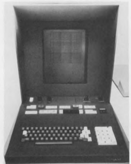
Interactive display terminal from Corning contains a photochromic CRT. A superimposed slide is shown on the screen.
