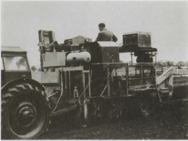
Instant evaluation of an experimental potato picker is done by a minicomputer at the Institute of Agriculture, Edinburgh, Scotland.
