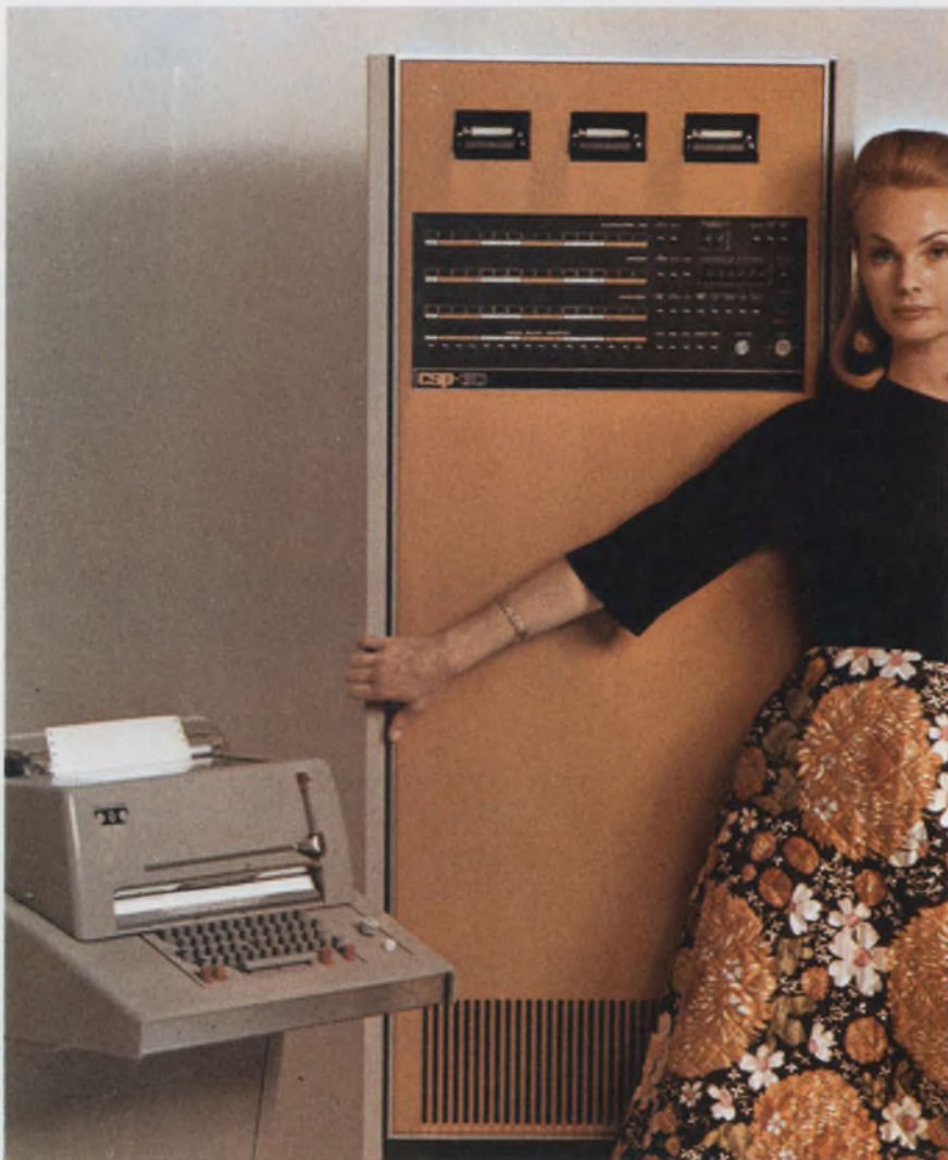
Using a combination memory of ICs and cores, a new low-cost high-speed 16-bit digital computer features a basic cycle time of 100 ns.
