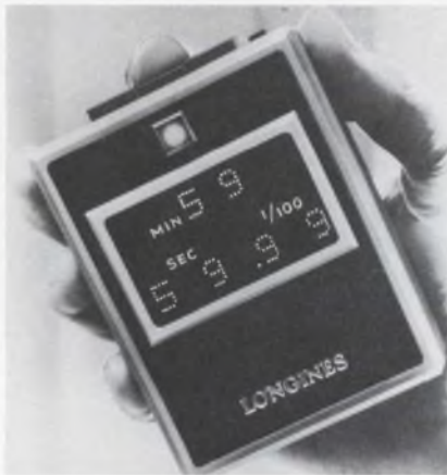
The basic technology for the wristwatch of the future is incorporated in this quartz-crystal stopwatch for sports, using solid-state displays.
