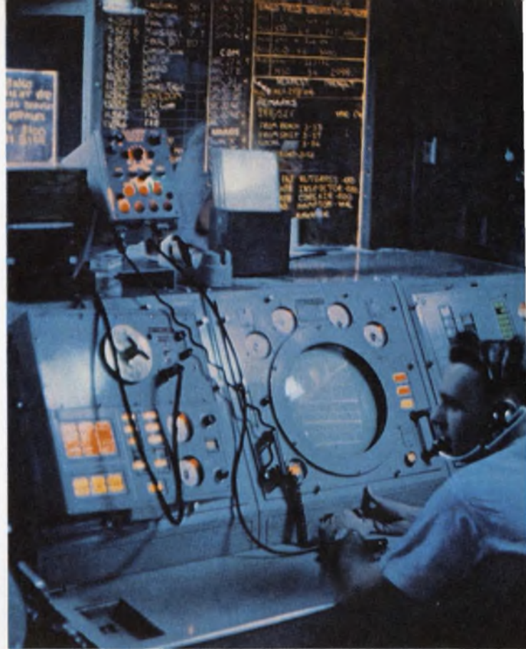
Shipboard SPN-10 radar operator watches and gives corrections for pilot's glide-slope and azimuth errors.
