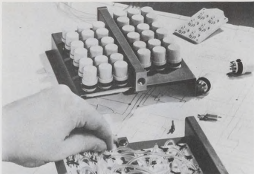
NOR impact modulator elements assembled to form a fluidic control circuit. Plastic tubing connects the logic elements.
