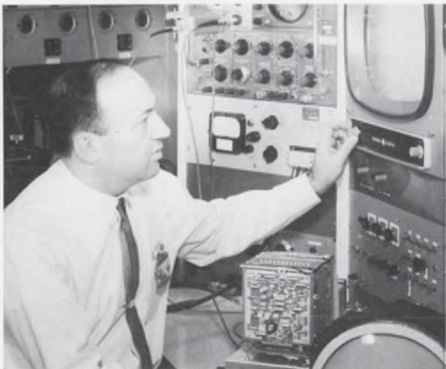
Author Hildebrant about to test the linearity of a magnetic deflection system.
