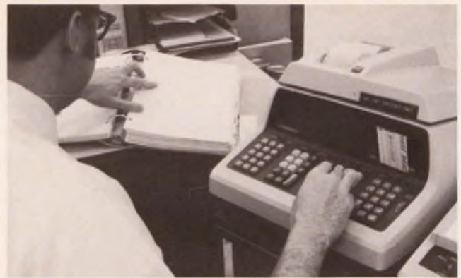
5. Magnetic card is one method by which programs can be entered into the calculator.
