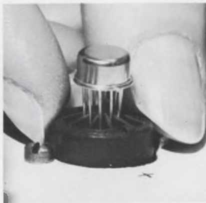
Ion-implanted 64-bit dynamic MOS shift register can clock at rates as fast as 20 MHz.
