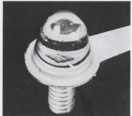
Ion-implanted 64-bit dynamic MOS shift register can clock at rates as fast as 20 MHz.
