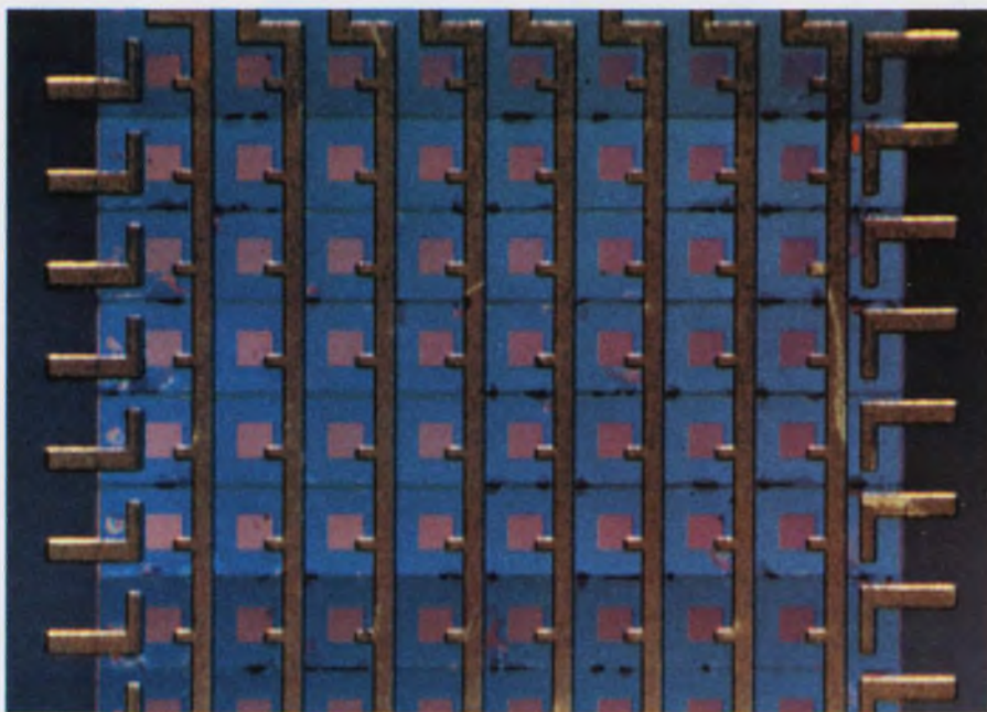
Holographic memories, such as this experimental Bell Laboratories model, promise storage densities of 10^8 bits per square inch.
