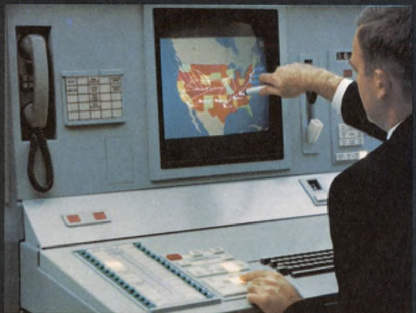
Light pen moves data on map overlay on Bunker-Ramo's BR-90 computer display terminal.
