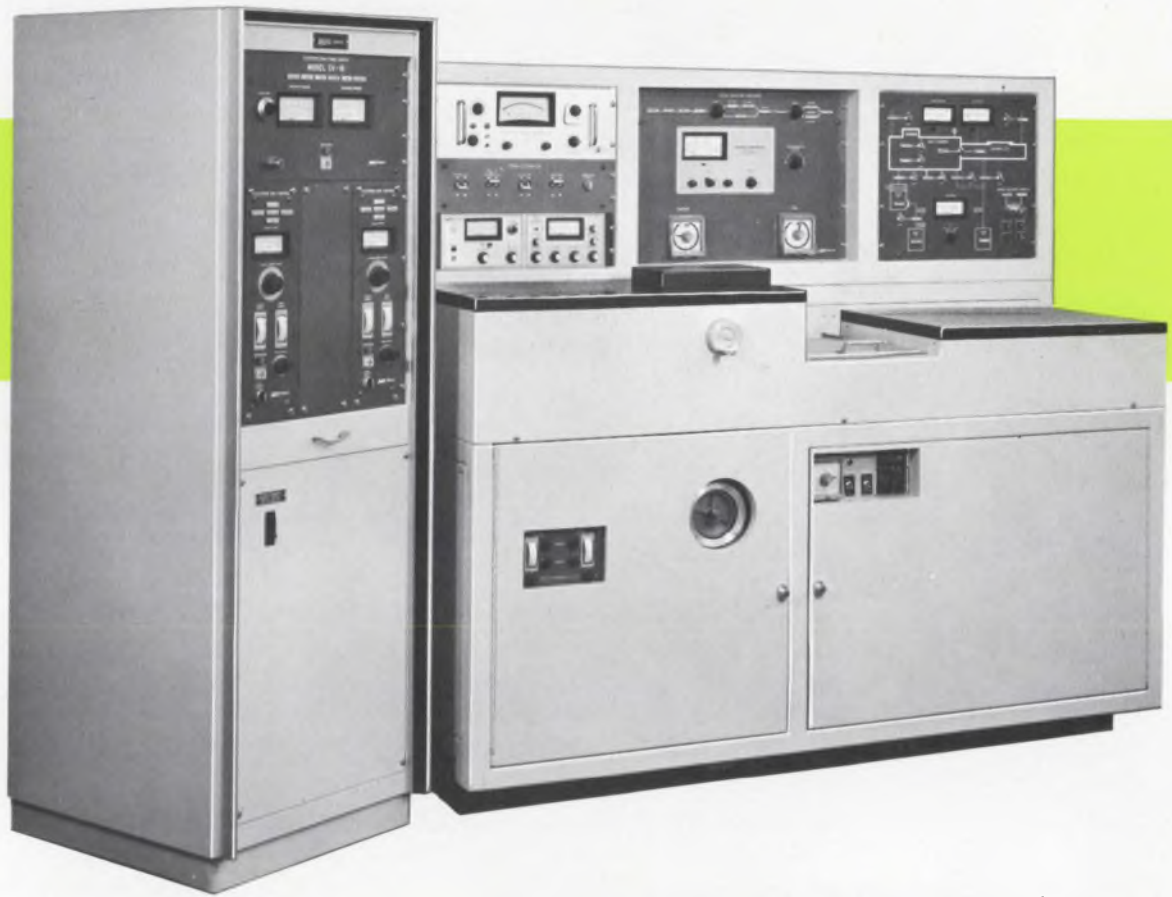
General Electric meters, SCRs, capacitors, selector switches, indicating lights, Volt-Pacs®, gear motors, current transformers and arc pilot devices are used in Airco Temescal's line of Integrated Electron Beam Systems and products such as this Thin-Film Electron Beam Deposition System. (For more information, circle 811.)
