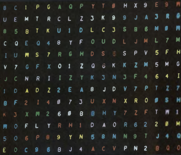
Chart used to test color and resolution of images for large-screen displays at Rome Air Development Center.
