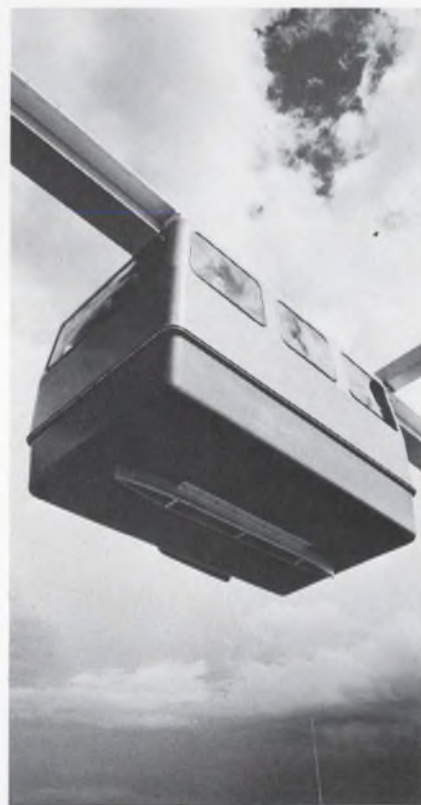
Computer-run monorail being readied for airport service. The Varo Monocab is a reinforced, molded fiberglass vehicle that will comfortably seat six passengers and has space for luggage. Air conditioning, thermal insulation and sound-proofing are featured. It will go into service at the new Dallas-Fort Worth Regional Airport.
