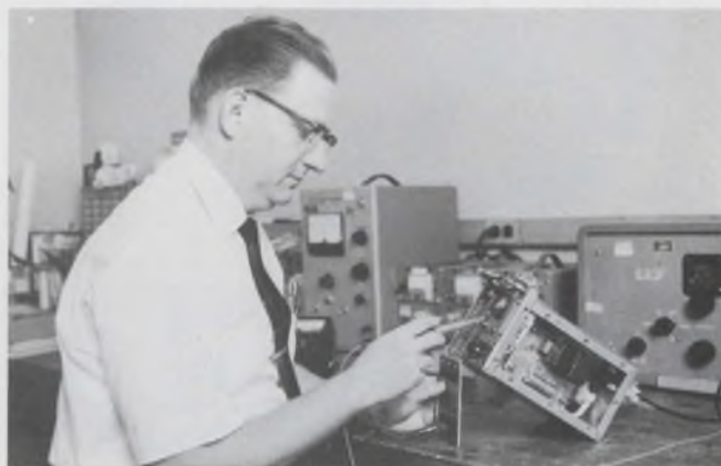
Author F. H. Wolf, in his laboratory, is testing the portion of the system containing the afc circuits.
