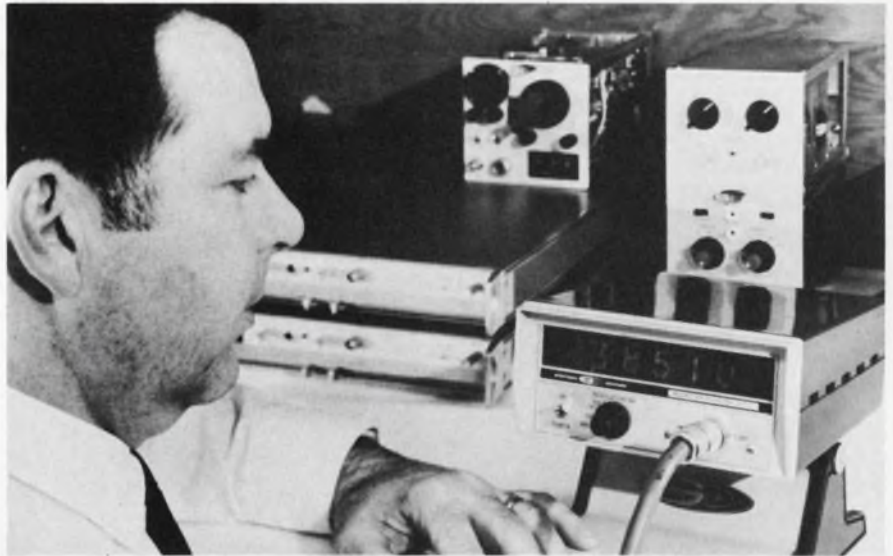
Miniature microwave counter by Systron-Donner counts from 300 MHz to 3 GHz. It will be on display at booth 1412.
