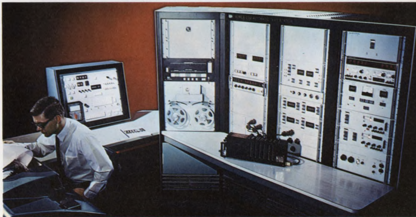
Computer-controlled test system from Bendix Corp. automatically checks on the performance of analog, digital
