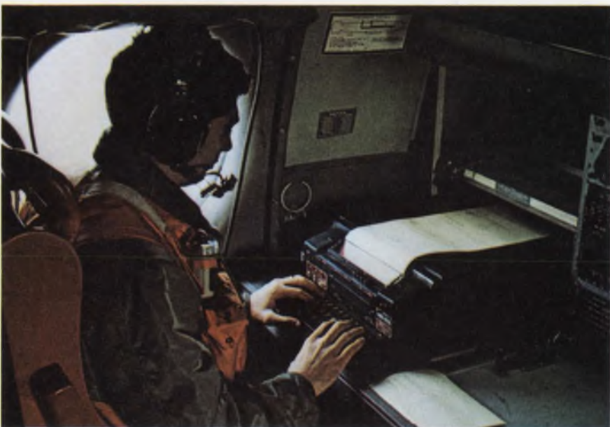
Radio operator on P-3 Orion can send teletypewriter messages over two AN/ARC-94 high-frequency transceivers.
