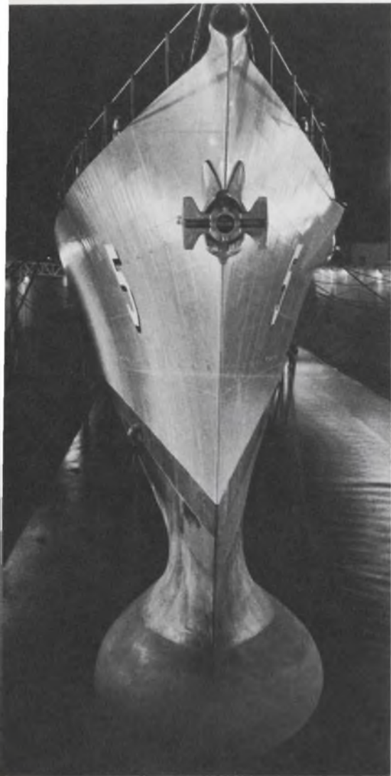
Biggest hull-mounted sonar in the fleet is the AN/SQS-26, built by GE.
