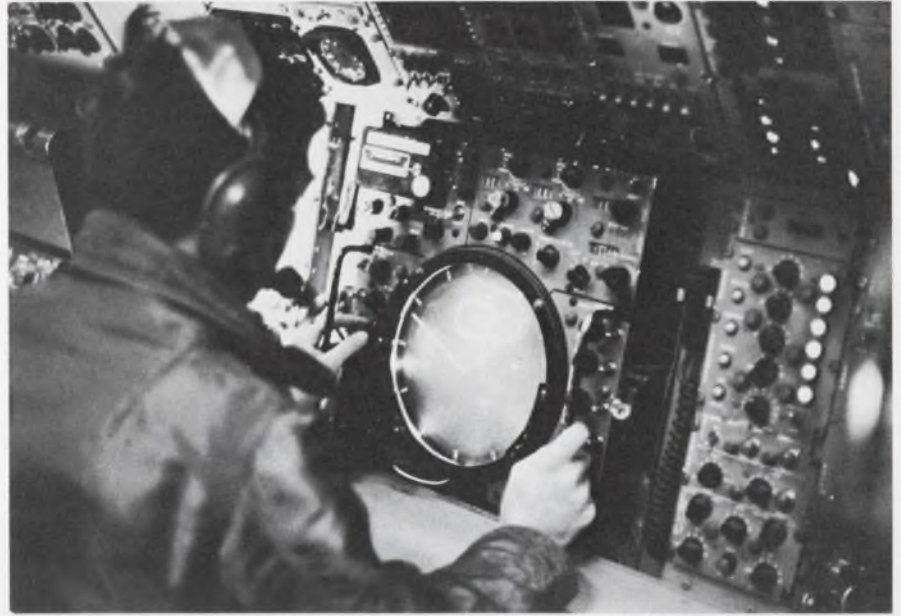
Tactical coordinator in a patrol plane, the P-3 Orion, watches the computerized display on his AN/ASA-16 indicator for sonobuoy positions and signals. Circles show sonobuoy range, while straight lines show range and bearing. The Orion is the Navy's newest land-based ASW aircraft.
