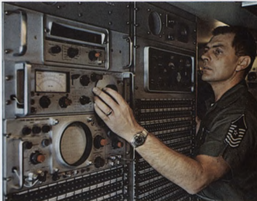
Technical control van provides quality control for all circuits leaving a center, plus retransmitting doubtful channels on another band.
