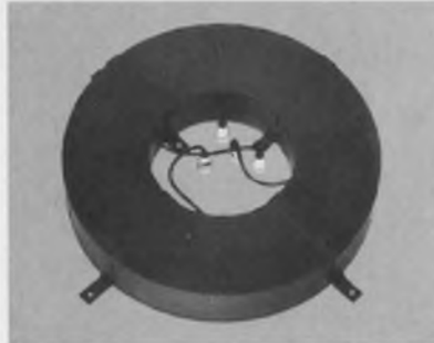
Dual section potted delay line. Outer race accounts for 980 nanoseconds; an inner nest exhibits 61.1 nanoseconds of delay. 50 ohm coaxial cable .215" diameter. Weight is 25 pounds for the 16" diameter, 3" high package.
