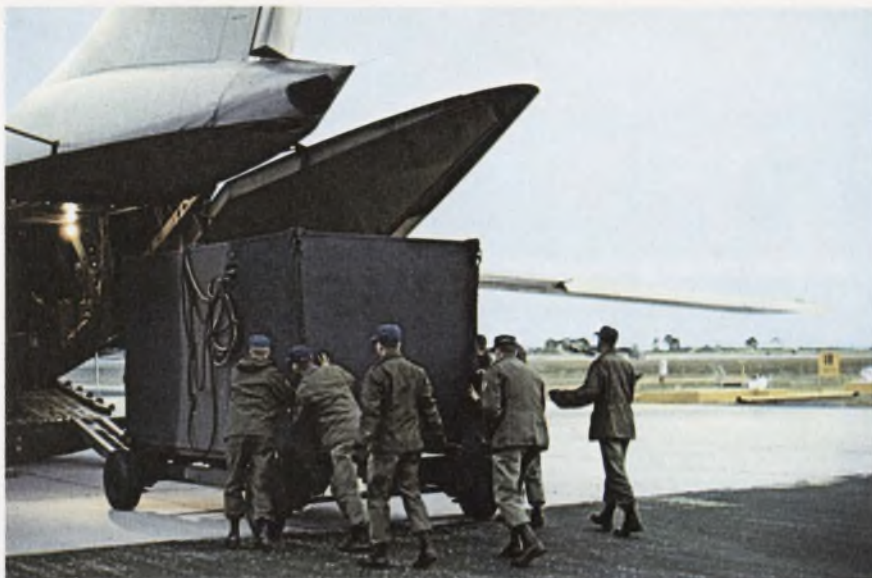
Jack Pot communications-relay/command-control system is rolled into C-141 transport jet for flight to Korea. On arrival its four vans, weighing 12 tons, will be put on a specially configured C-130 for the flight.
