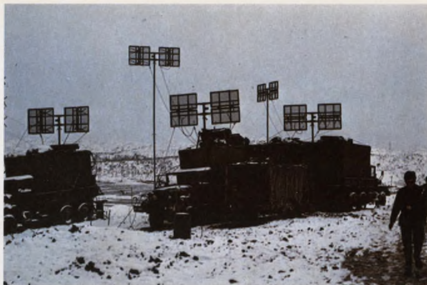
Communications headquarters for the entire Focus Retina exercise were set up on five hills alongside the command center. Waffle-like antennas reveal the old vhf AN/TRC-24 radio as still the Army's workhorse.
