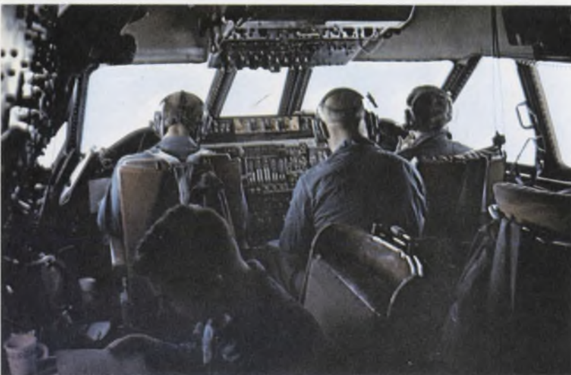
C-141 transport jet that flew troops and equipment to South Korea is getting all-weather landing system that permits hands-off touchdown.
