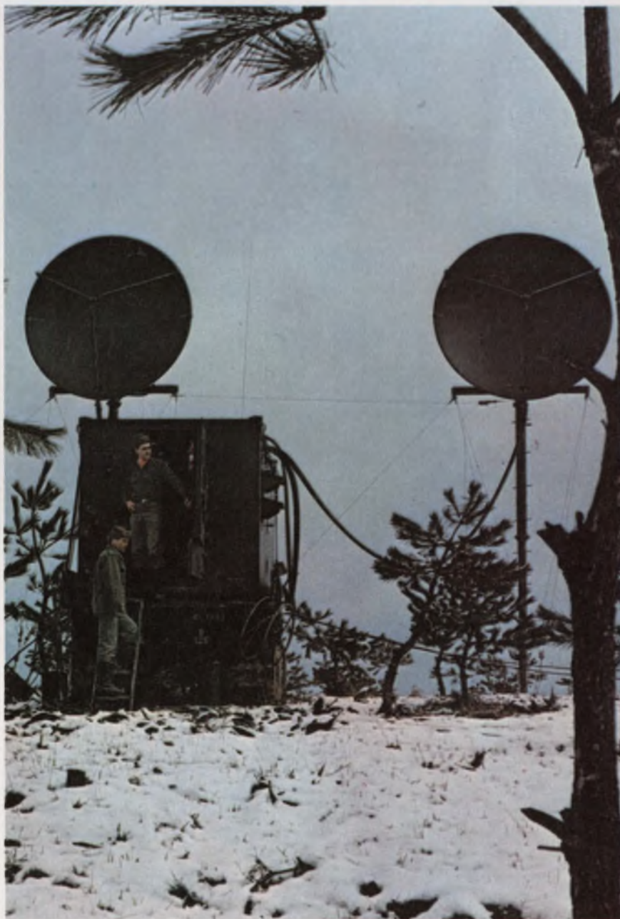
The Army in Korea favors tropo communications, like this TRC-129A, over hf and vhf and wants to use it over shorter distances. "This can be done," Collins Radio says, "with more work on the electronic combining function."
