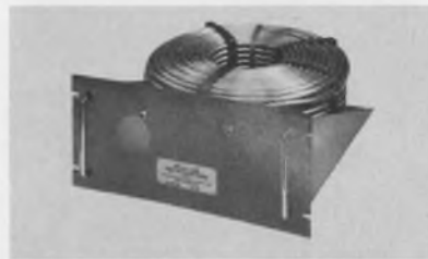
Standard delay line for calibration of oscilloscopes, altimeters, radar systems and similar applications. Measures 8 1/2" x 21" x 19", offers a delay of 500 nanoseconds, calibrated to \pm 0.25 nanoseconds.
