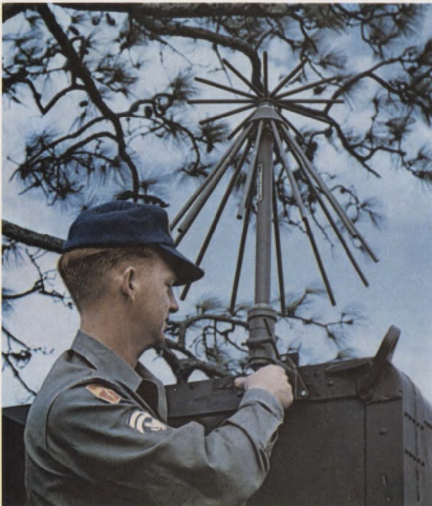
Non-directional discone antenna rises above one of five air-transportable satellite communications terminals built and ready for use by the Air Force at MacDill AFB, Fla., with the aid of Electronic Communications, Inc.
