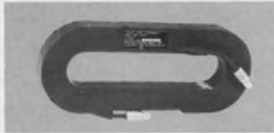
Encapsulated delay line, used between 8 and 12 Gc, exhibits 100 nanoseconds of delay. Weighs less than 8 pounds, cable is 70 feet long, .270" diameter, 50 ohm impedance.
