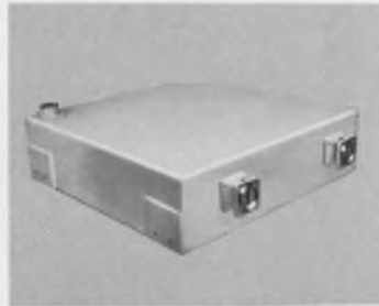
KU band delay line exhibits loss of less than 30 DB with maximum of 1:3:1 at 13 GHz. Built-in thermal insulation and solid state temperature control. Internal waveguide to coax transitions.
