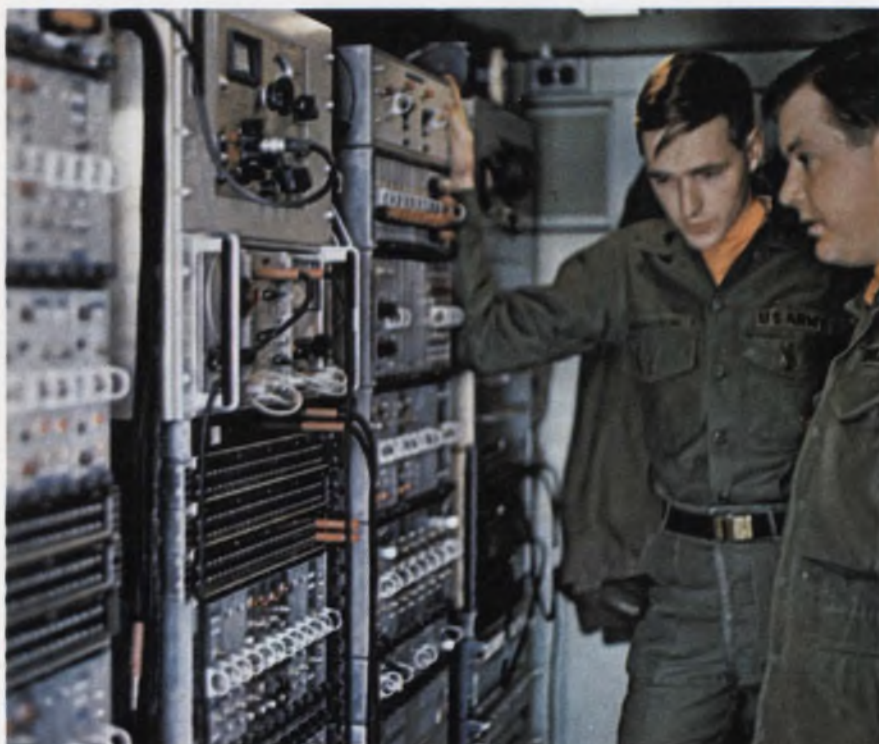
Van for tropo communications, AN/TRC-129A, sits on 2-1/2-ton truck in Korea. It's a little bigger than similar units to provide an hf radio, a teletypewriter and more room for the operators, Collins Radio says.
